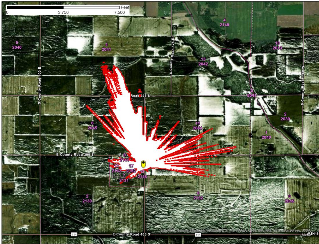
Figure 1 – Mount Ayr, IN SAN -77.6 \text{ dB(mW/(m}^2 * \text{MHz))} pfd contour
