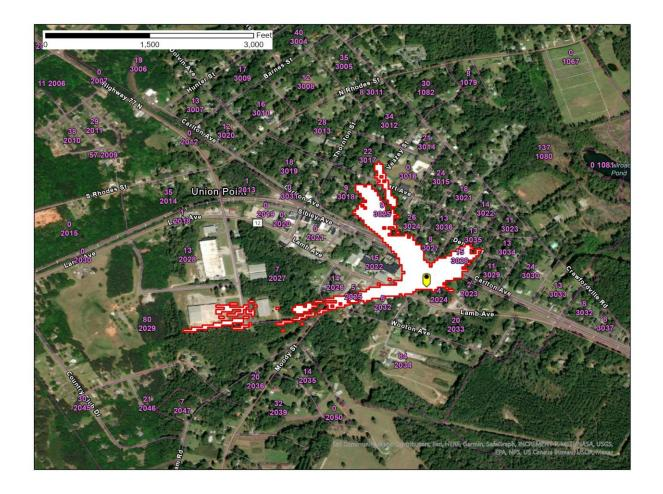
Figure 1 – Union Point, GA SAN -77.6 dB(mW/(m2 \* MHz)) pfd contour
