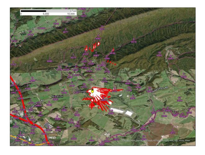
Figure 1 – Wytheville, VA SAN -77.6 dB(mW/(m2 \* MHz)) pfd contour
