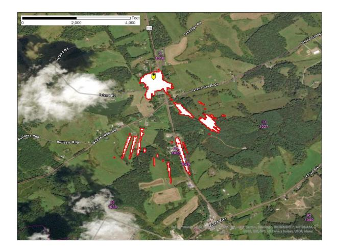
Figure 1 – Hillsville, VA SAN -77.6 dB(mW/(m2 \* MHz)) pfd contour
