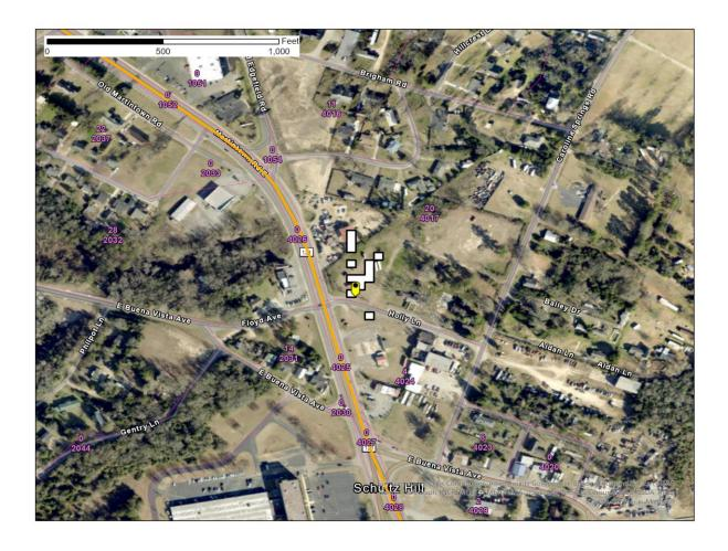
Figure 1 – North Augusta, SC SAN -77.6 dB(mW/(m2 \* MHz)) pfd contour
