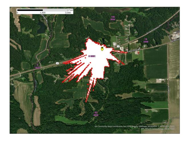
Figure 1 – Marshall, IL SAN -77.6 dB(mW/(m2 \* MHz)) pfd contour
