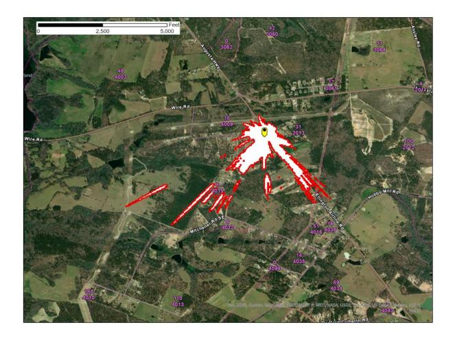
Figure 1 – Dearing, GA SAN -77.6 dB(mW/(m2 \* MHz)) pfd contour
