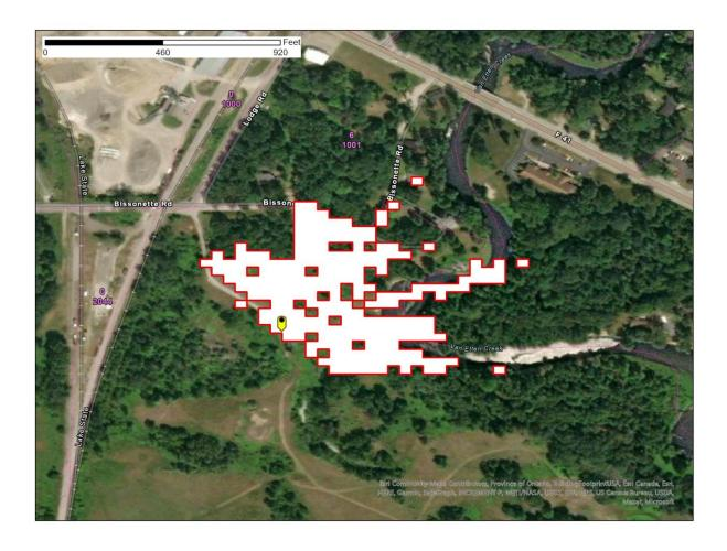
Figure 1 – East Tawas, MI SAN -77.6 dB(mW/(m2 \* MHz)) pfd contour
