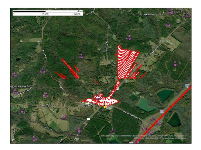
Figure 1 – Fosters, AL SAN -77.6 dB(mW/(m2 \* MHz)) pfd contour
