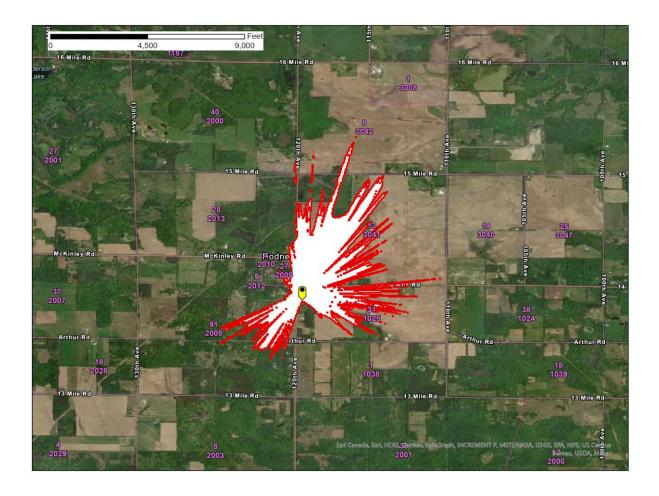
Figure 1 – Rodney, MI SAN -77.6 dB(mW/(m2 \* MHz)) pfd contour
