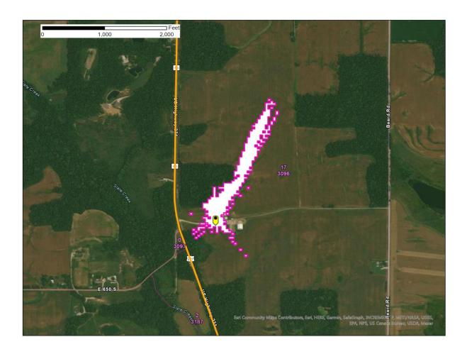
Figure 1 – Loogootee, IN SAN -77.6 dB(mW/(m2 \* MHz)) pfd contour
