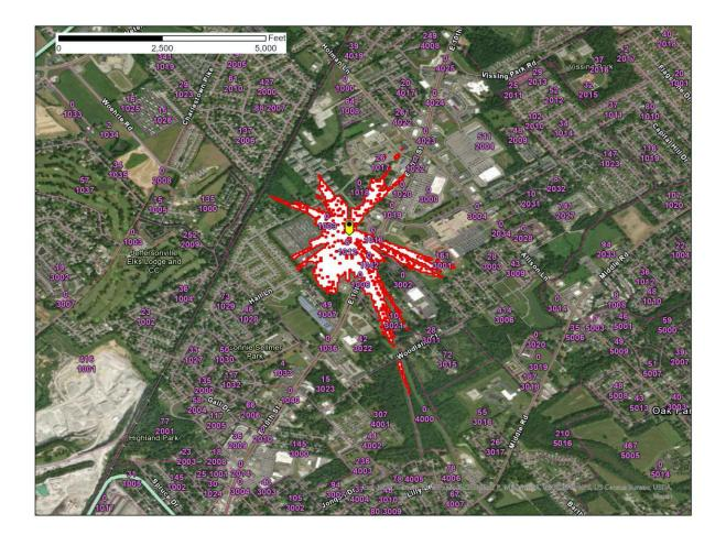
Figure 1 – Jeffersonville, IN SAN -77.6 dB(mW/(m2 \* MHz)) pfd contour
