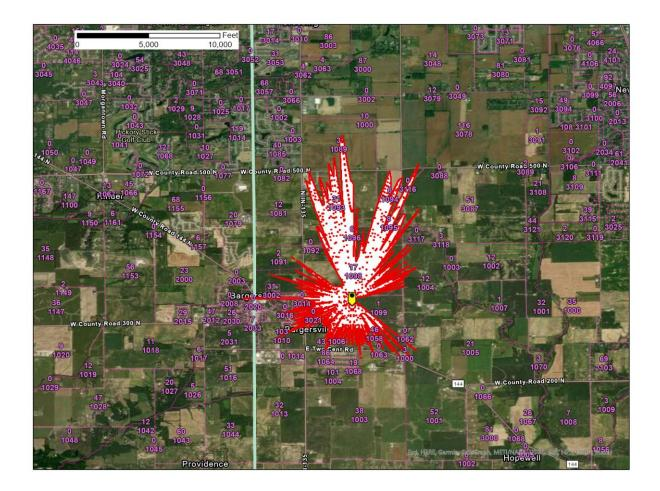
Figure 1 – Franklin, IN SAN -77.6 dB(mW/(m2 \* MHz)) pfd contour
