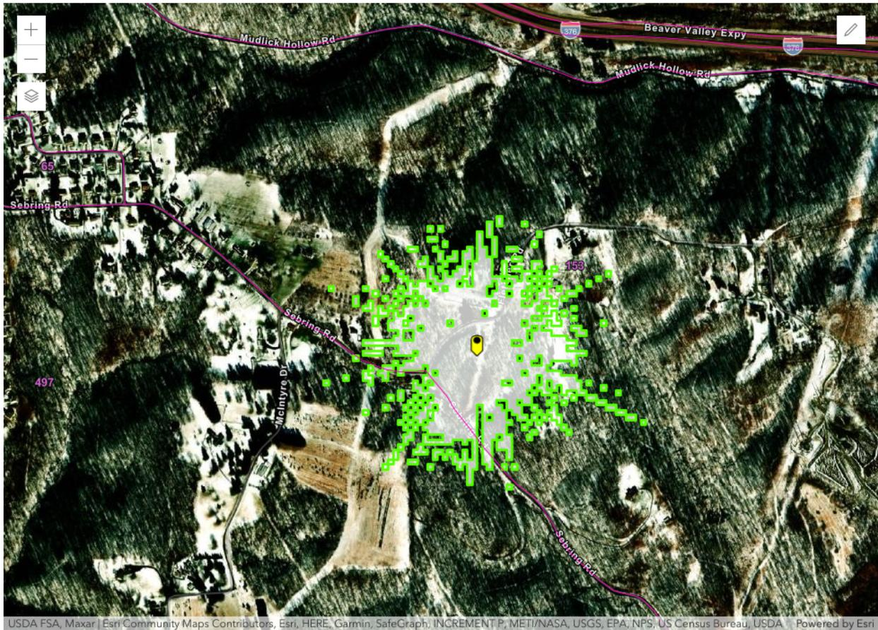
**Figure 1 – Beaver, PA SAN -77.6 dB(mW/(m<sup>2</sup> \* MHz)) pfd contour**
