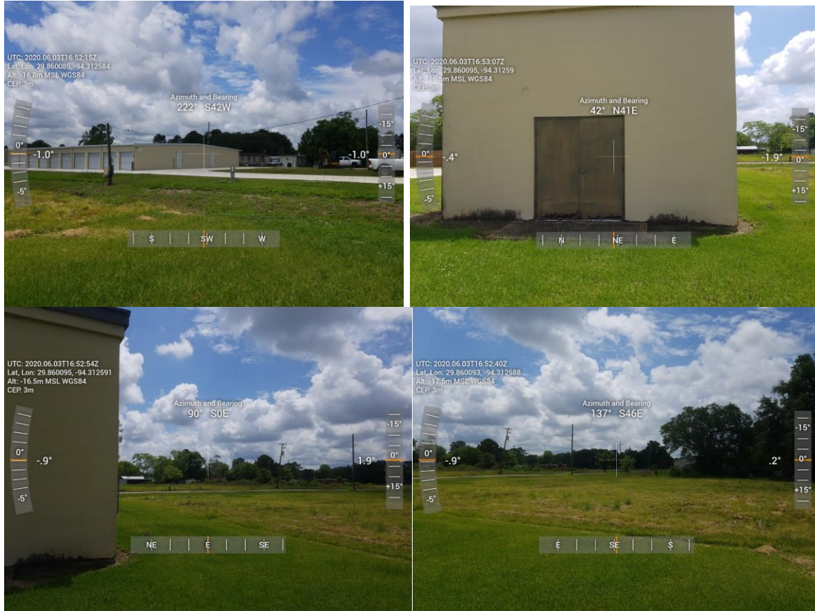
Figure 9: Photo of surroundings at earth station location in Hamshire, TX (Callsign E202201), obtained during in-person site survey. These images indicate that clutter assumptions used (4 meters height and 0.4 kilometers distance) are conservative. Based on the photos and measurements taken during in-person survey, tree and building heights exceed 4 meters in height and are less than 0.4 kilometers from the gateway location.
