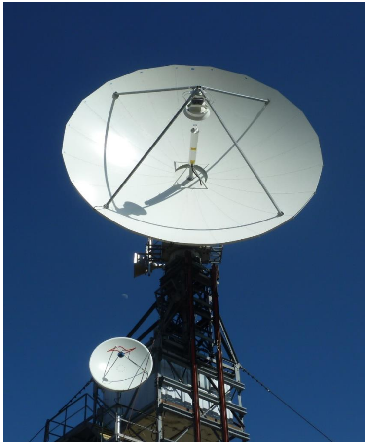
Figure 1: ASC 9.4m reflector antenna installed for testing.
