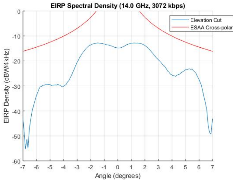
Figure 3-7 Cross-polarized Off-Axis EIRP Density in the plane perpendicular to GSO Arc (14.0 GHz)
