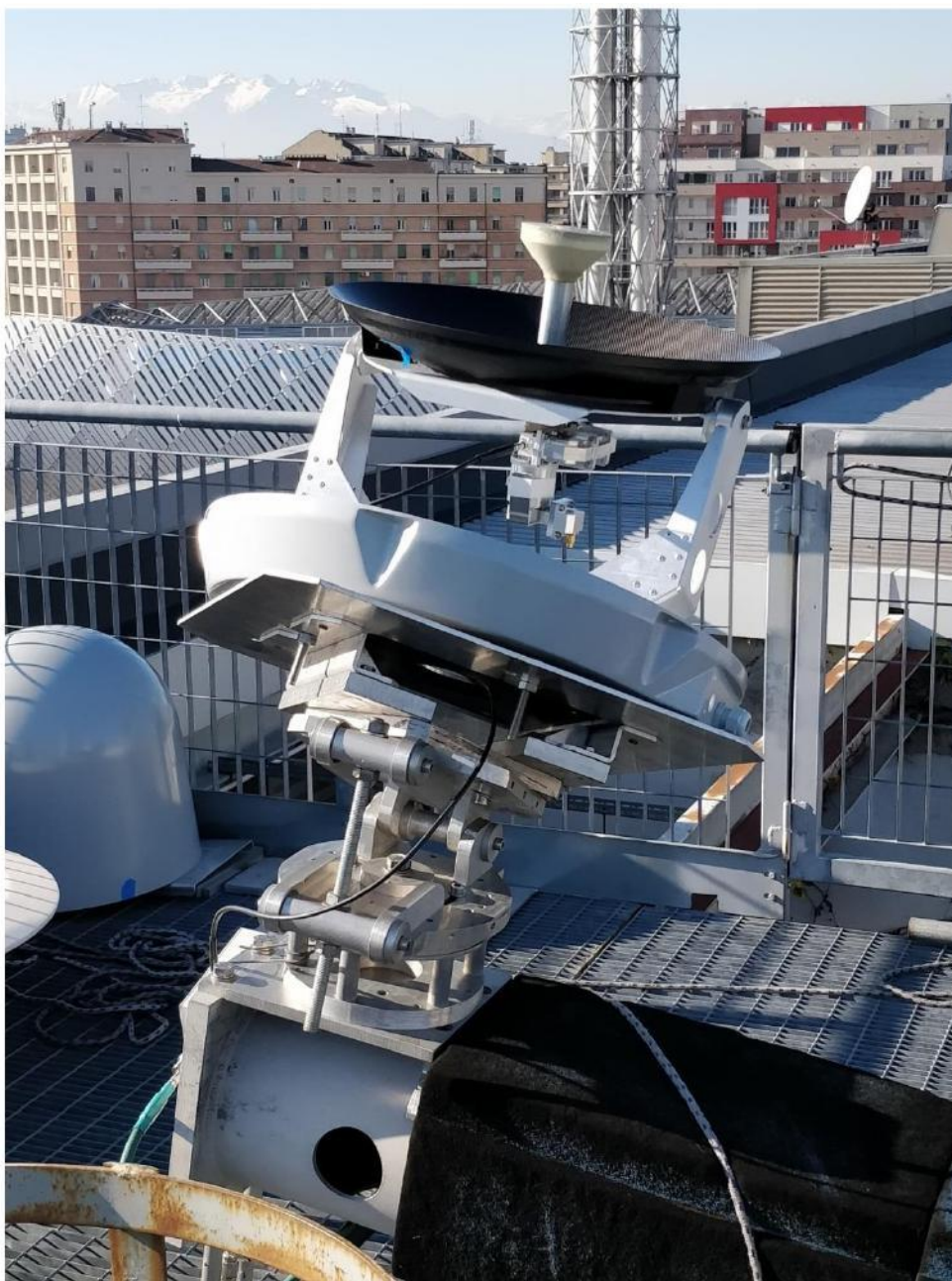
Fig.5: Antenna BB45Ku mounted on AUT positioner.
