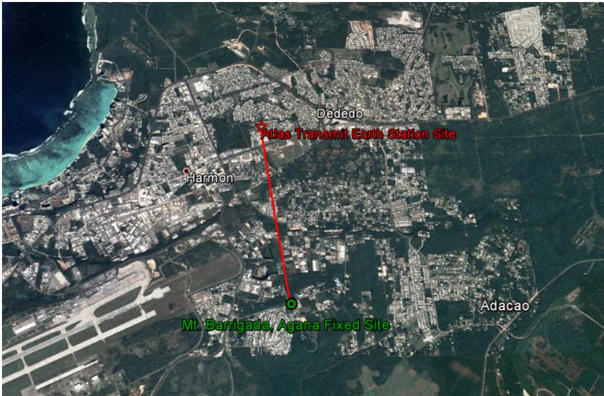
Figure 1 – Atlas E/S site and GERP Broadcast Auxiliary Remote Pickup Fixed Site. Remote pickups within 19km of Fixed site.
