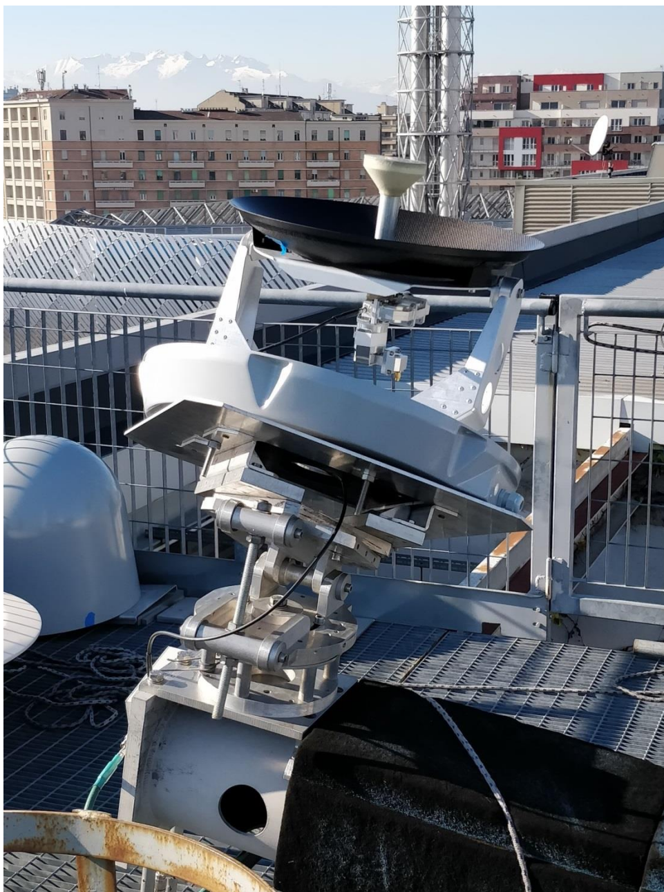
Fig.5: Antenna BBIG45Ku mounted on AUT positioner.
