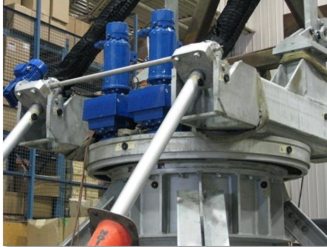
FIGURE 9 VIEW OF AZIMUTH DRIVE
