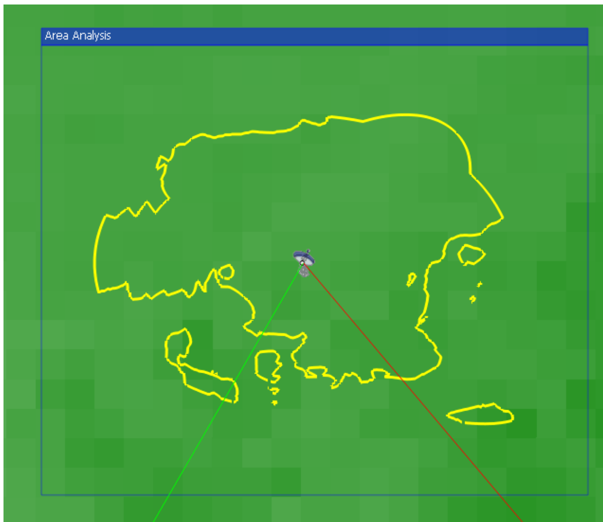
Fig A.12.3. C/I contour of 23.2 dB with Rec 580 pattern for Gateway Station (BSS feeder link antenna pointed towards BSS satellite at 119.2 W.L.)
