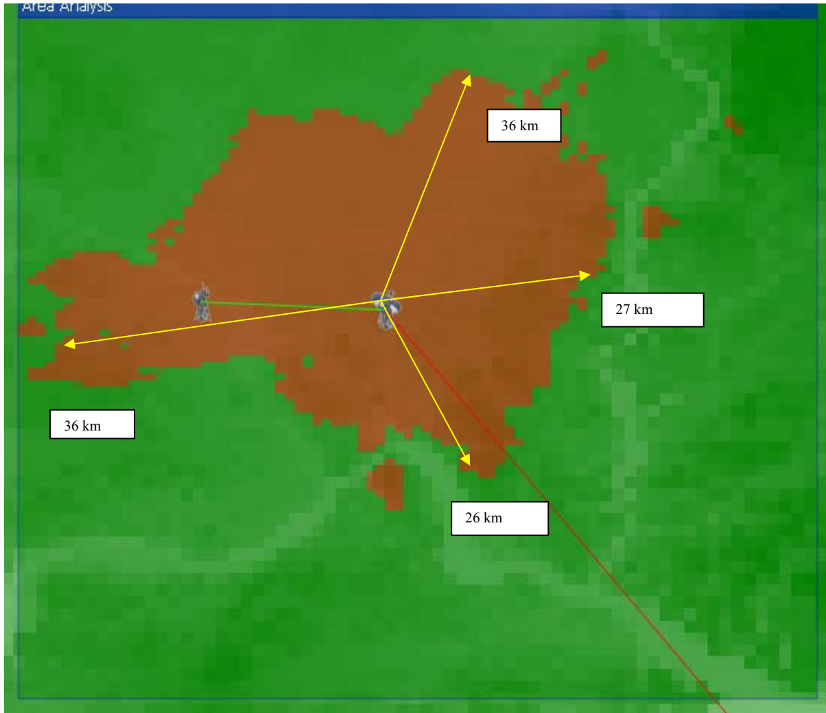
Fig A.13.1. Required C/I criterion (23.2 dB) contour (Case A)
