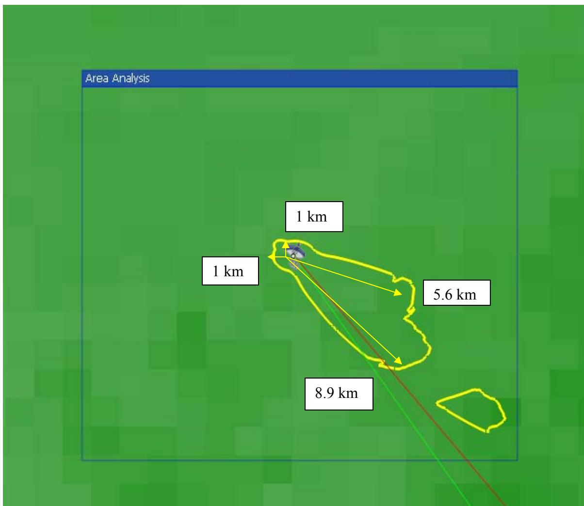
Fig A.12.2. C/I contour of 23.2 dB with the measured antenna pattern for Gateway Station (BSS feeder link antenna pointed towards BSS satellite at 61.5 W.L.)
