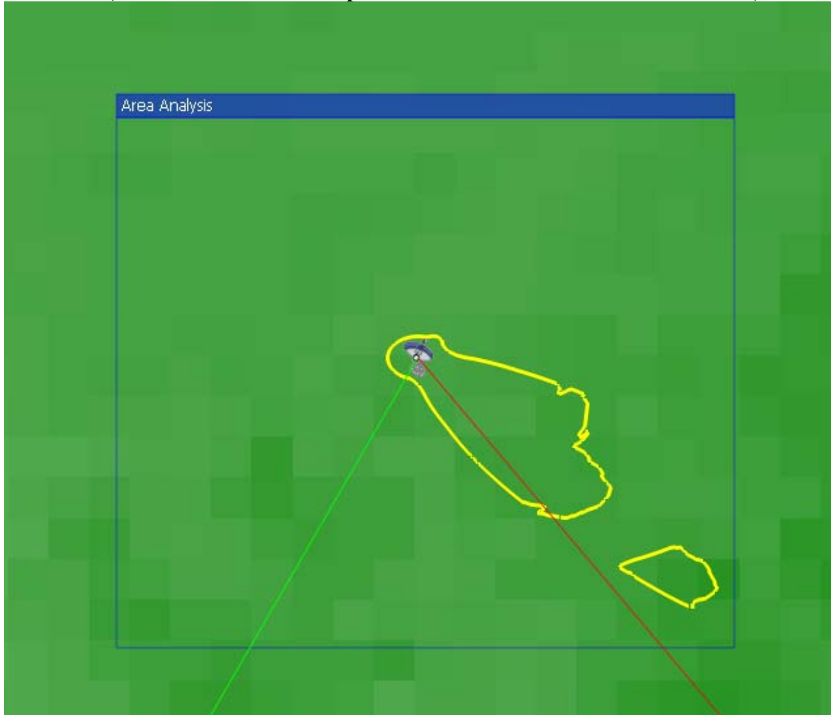
Fig A.12.4. C/I contour of 23.2 dB with the measured antenna pattern for Gateway Station (BSS feeder link antenna pointed towards BSS satellite at 119.2 W.L.)
