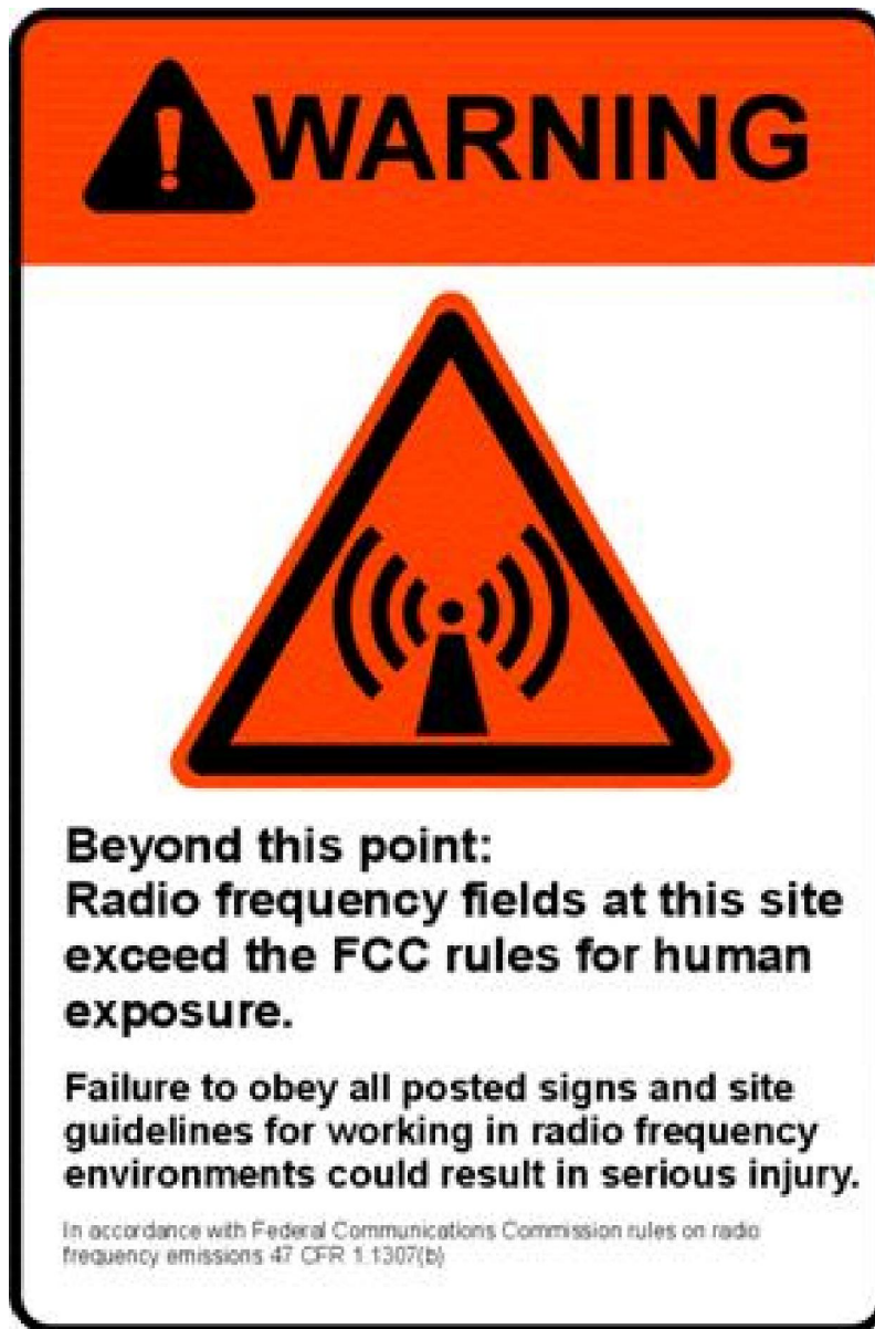
Figure 8 - Radiation Hazard Warning Label Sample
