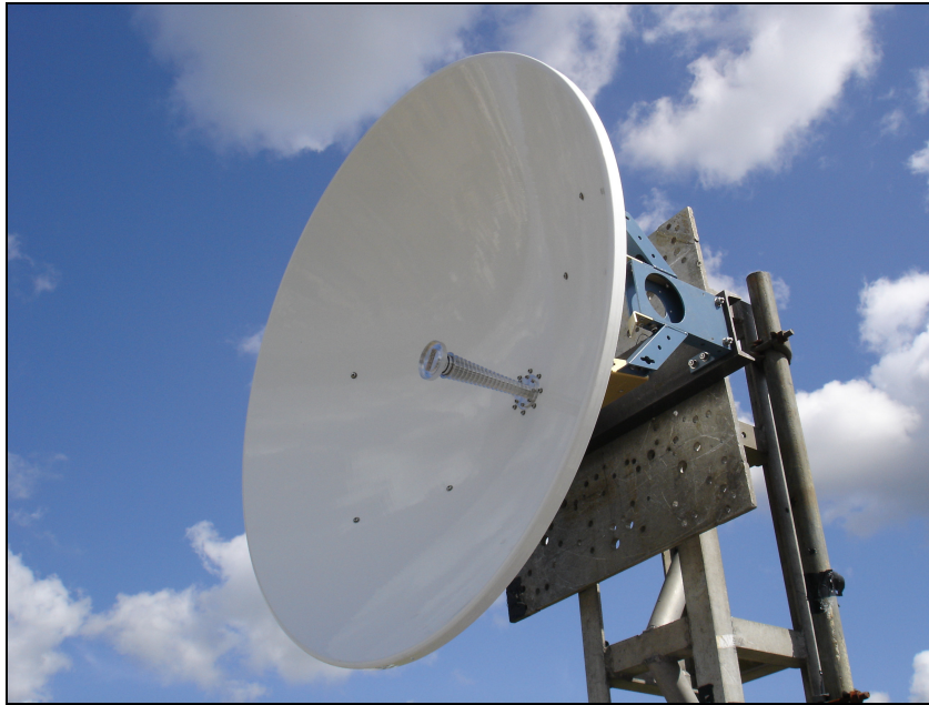
Figure 1: 1.0 metre Ku band reflector on ERA far field range
