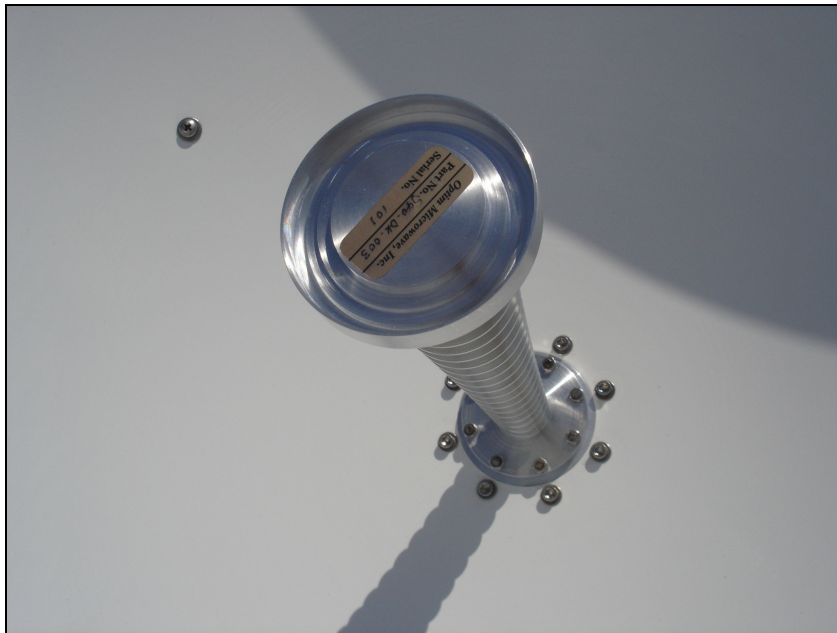
Figure 2: Detail of feed/subreflector combination of 1.0 metre Ku band reflector
