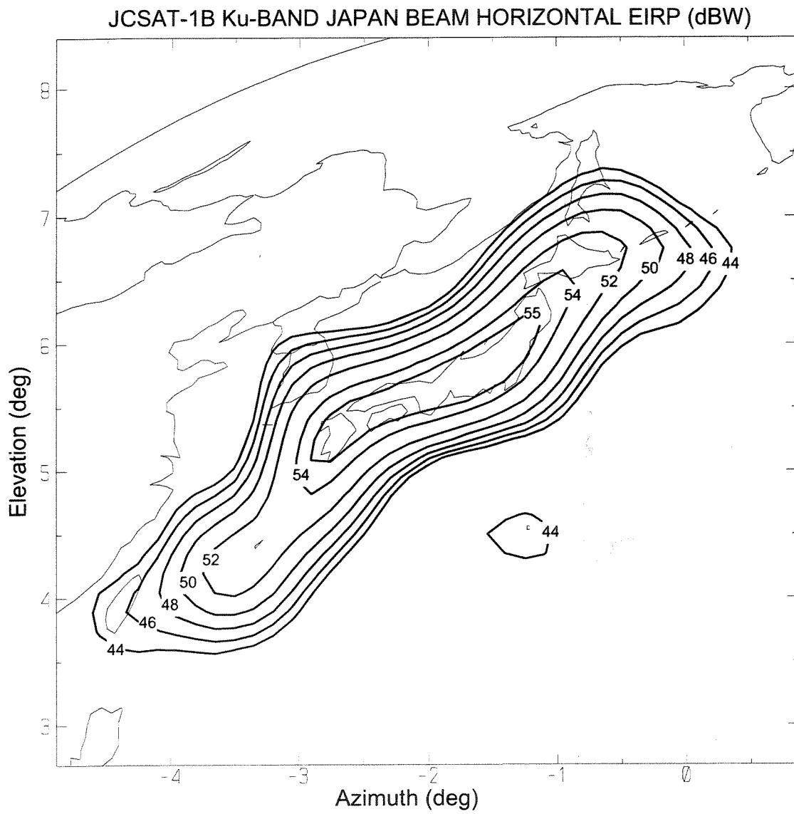
Note) JCSAT-1B EIRP shall be operated under 4.6dB backoff level
