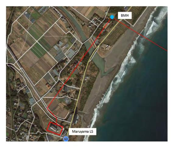
Beach manhole geographic coordinates: Latitude: N35 00.767 Longitude: E139 58.786 Cable landing station geographic coordinates: Latitude: N35 00.326 Longitude: E139 58.528 Cable landing station street address: 2698-19 Shirako, Minamibousou-shi, Chiba, Japan
