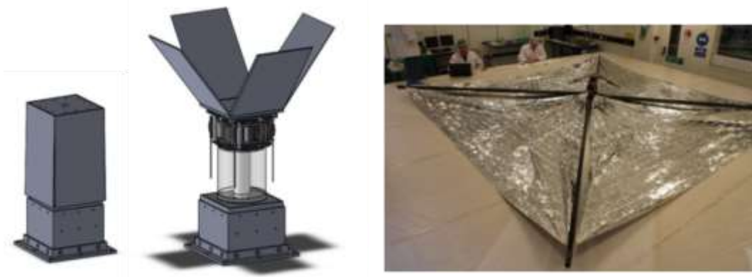
Figure 1: Deorbit Device in stowed configuration, deployed configuration, and the fully deployed sail.
