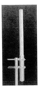
The TA-2350-DAB is a medium power vertically polarized omnidirectional antenna specifically designed for Digital Audio Broadcast transmission. The antenna consists of a phased corporately fed broadband dipole array which is configured to provide electrical beam downtilt and null fill. The antenna elements are at DC ground to aid in lightning protection.
