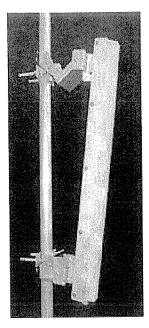
The TA-2304-2-DAB is a medium power vertically polarized sectoral antenna specifically designed for Digital Audio Broadcast transmission. The antenna is designed to provide field adjustable azimuth beamwidths of 45, 60, 90, 120, or 160 degrees by use of side panels. The antenna elements are at DC ground to aid in lightning protection.
