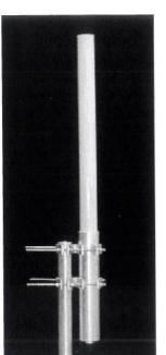
The TA-2350-DAB is a medium power vertically polarized omnidirectional antenna specifically designed for Digital Audio Broadcast transmission. The antenna consists of a phased corporately fed broadband dipole array which is configured to provide electrical beam downtilt and null fill. The antenna elements are at DC ground to aid in lightning protection.
