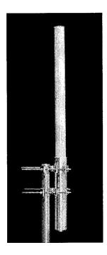
The TA-2350-DAB is a medium power vertically polarized omnidirectional antenna specifically designed for Digital Audio Broadcast transmission. The antenna consists of a phased corporately fed broadband dipole array which is configured to provide electrical beam downtilt and null fill. The antenna elements are at DC ground to aid in lightning protection.
