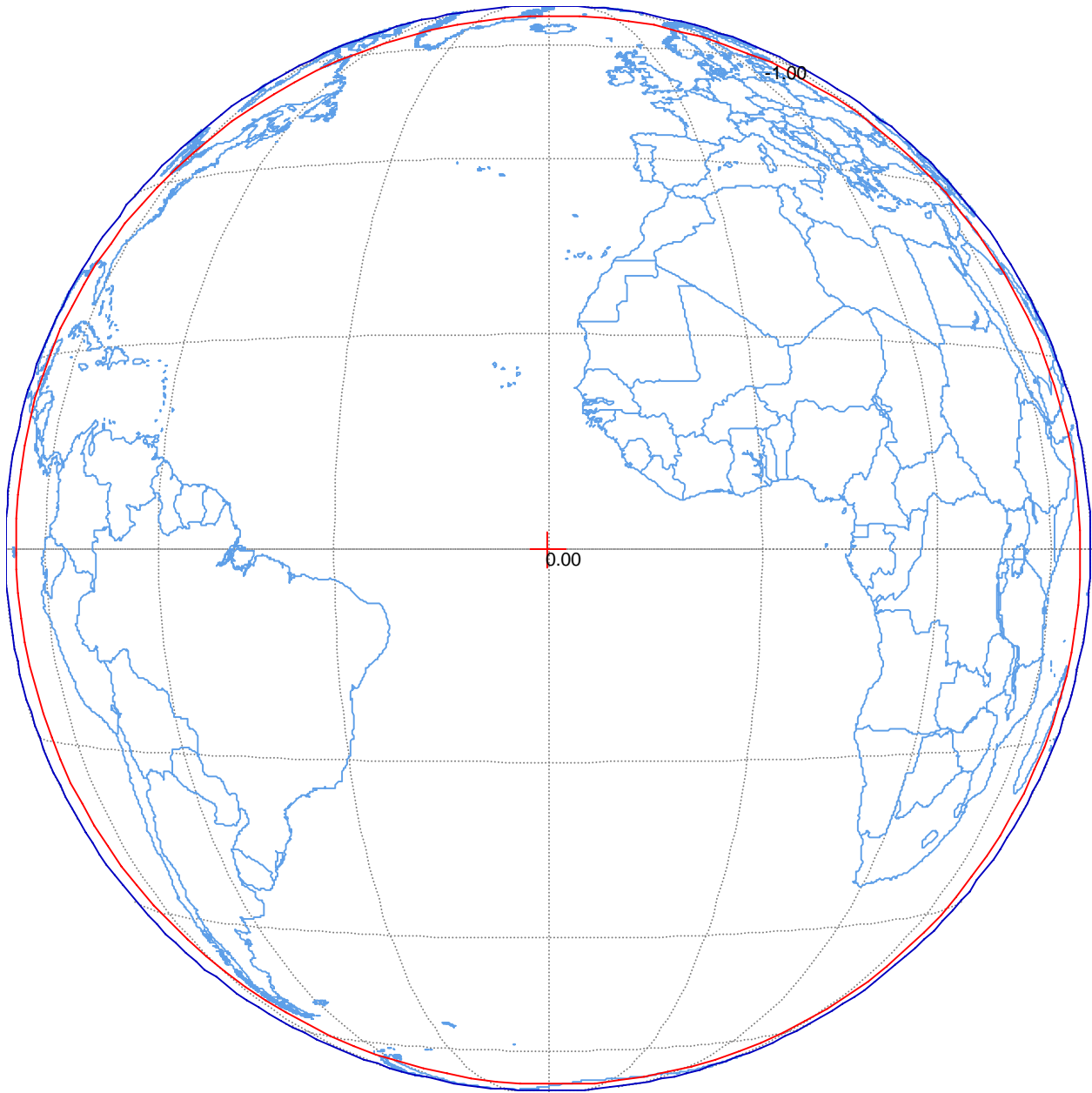
Figure B-15. Command Carrier Earth Facing Receive Horn 11 Maximum receive gain = 11 dBi Command Threshold Flux Density = -90 dBW/m 2 Polarization RHCP Schedule S beam designator: CMD
