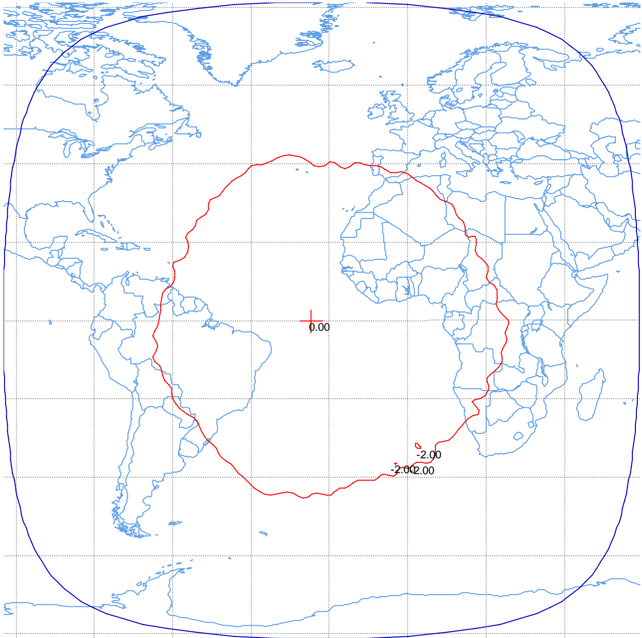
Figure B-2. Global Downlink Beam Peak EIRP = 36.6 dBW Peak Beam Gain = 20.9 dBi Polarization RHCP and LHCP Schedule S beam designators: GBAD and GBBD 10
