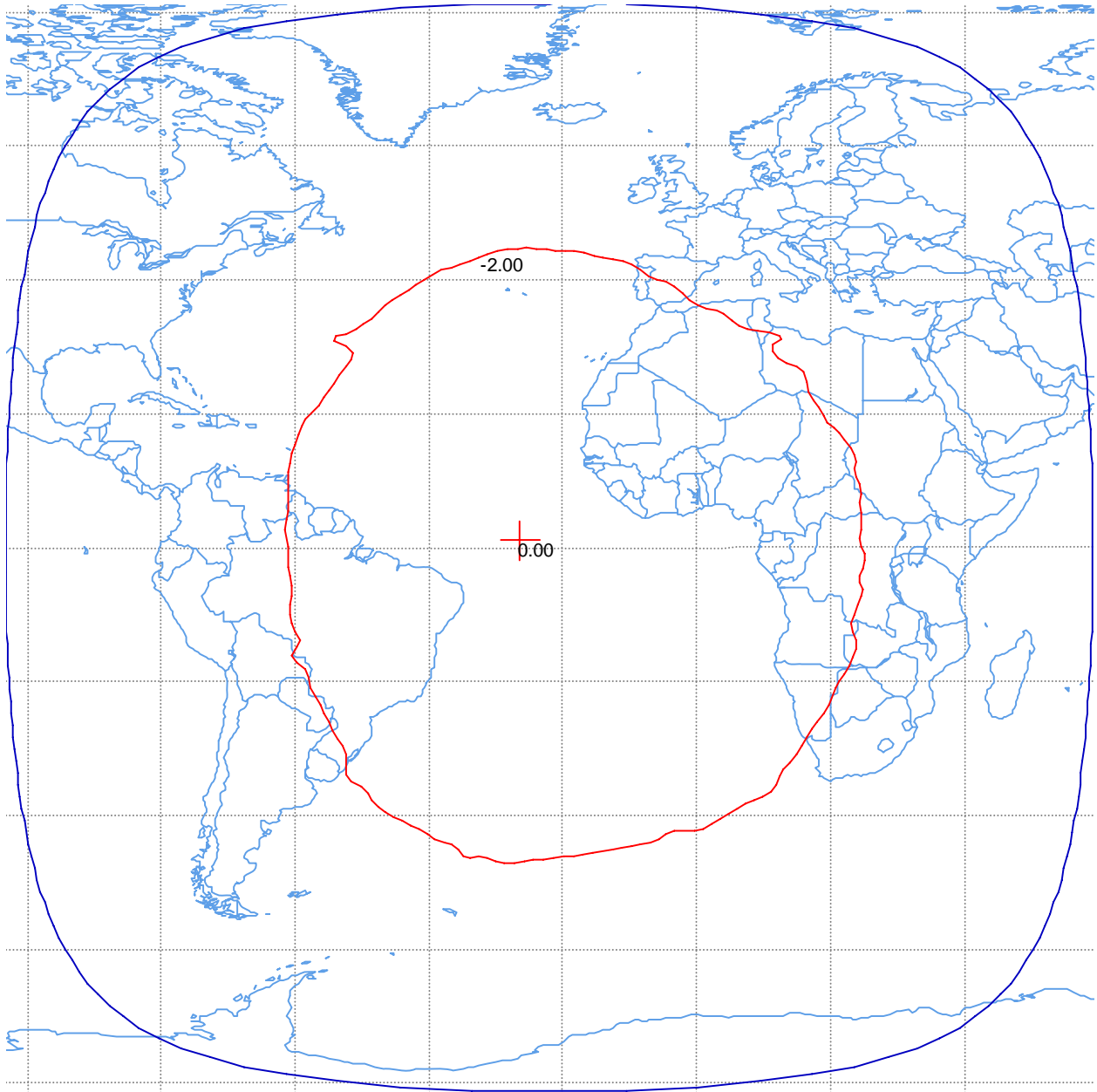
Figure B-1. Global Uplink Beam Peak G/T = -7.6 dB/K Peak Beam Gain = 20.9 dBi Min. Saturation Flux Density = -93 dBW/m 2 Polarization LHCP and RHCP
