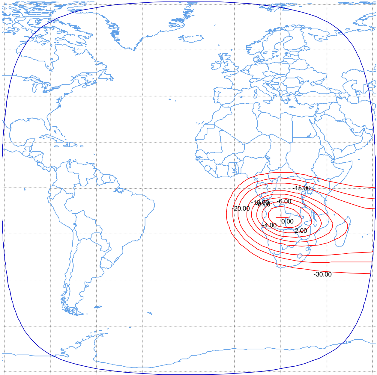
Figure B-17. Spot 1 Uplink Beam Peak G/T = 10.4 dB/K Peak Beam Gain = 39.4 dBi Min. Saturation Flux Density = -101 dBW/m 2 Polarization Vertical or Horizontal Linear Schedule S beam designators: S1AU and S1BU
