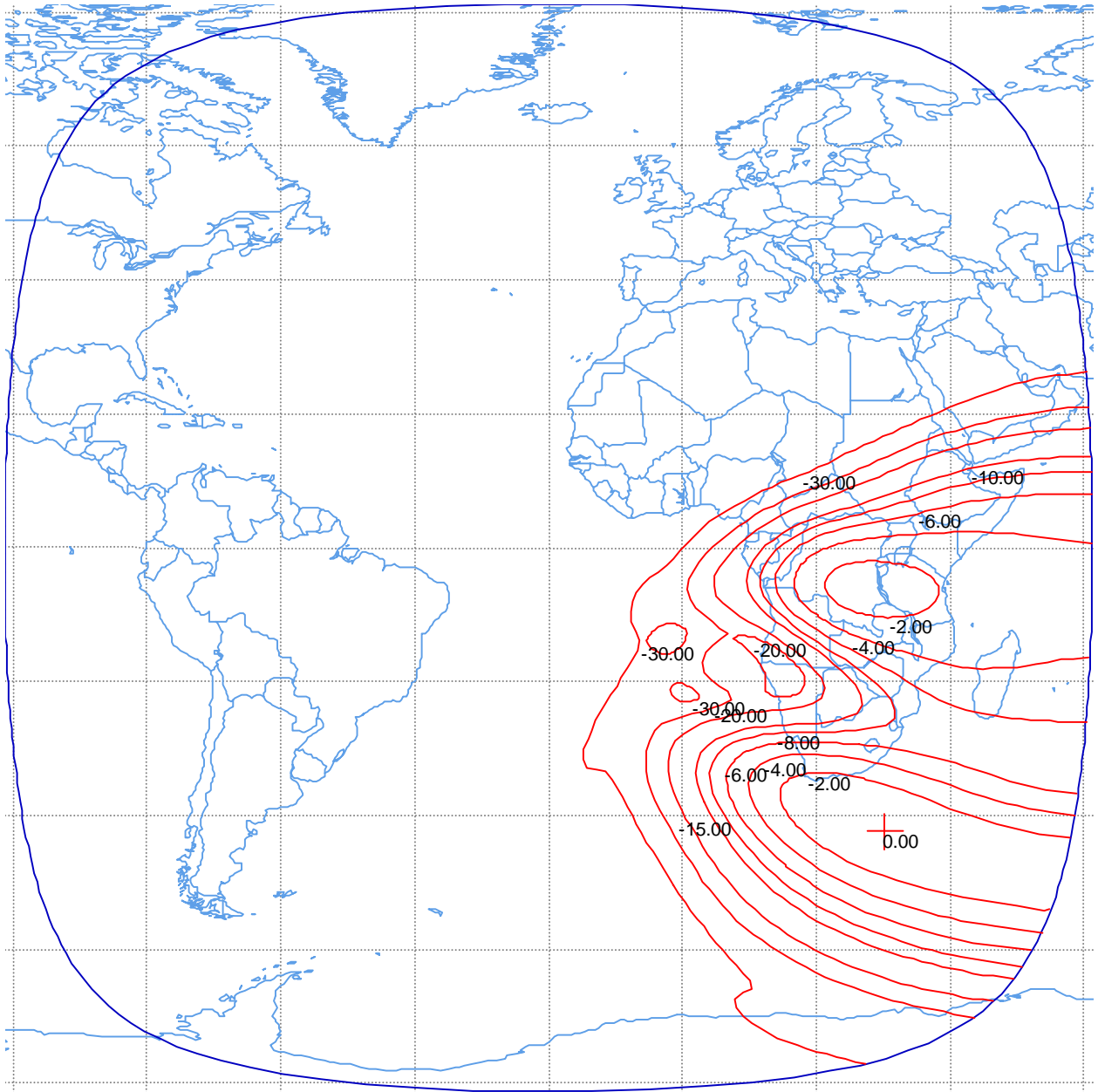
Figure B-13. South East Zone Uplink Beam Peak G/T = 2.2 dB/K Peak Beam Gain = 30.9 dBi Min. Saturation Flux Density = -96 dBW/m 2 Polarization RHCP Schedule S beam designator: SEZU
