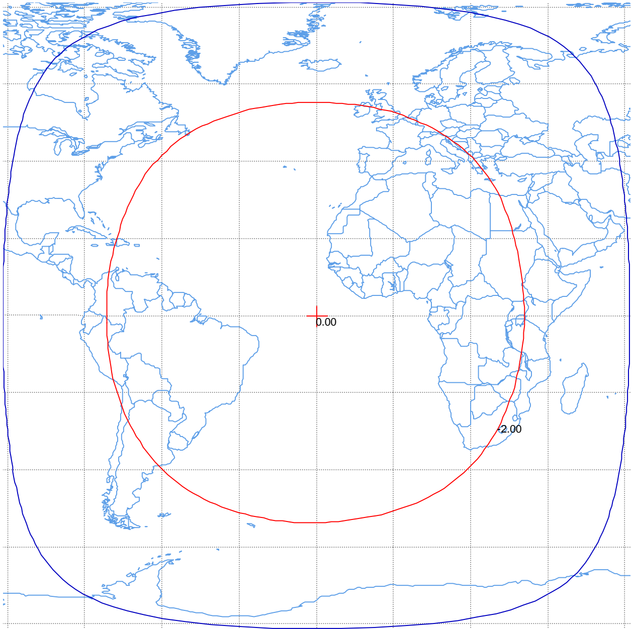
Figure B-1. Global Uplink Beam Peak G/T = -8.4 dB/K Peak Beam Gain = 20 dBi Min. Saturation Flux Density = -92 dBW/m 2 Polarization LHCP and RHCP Schedule S beam designators: GAU and GBU 10
