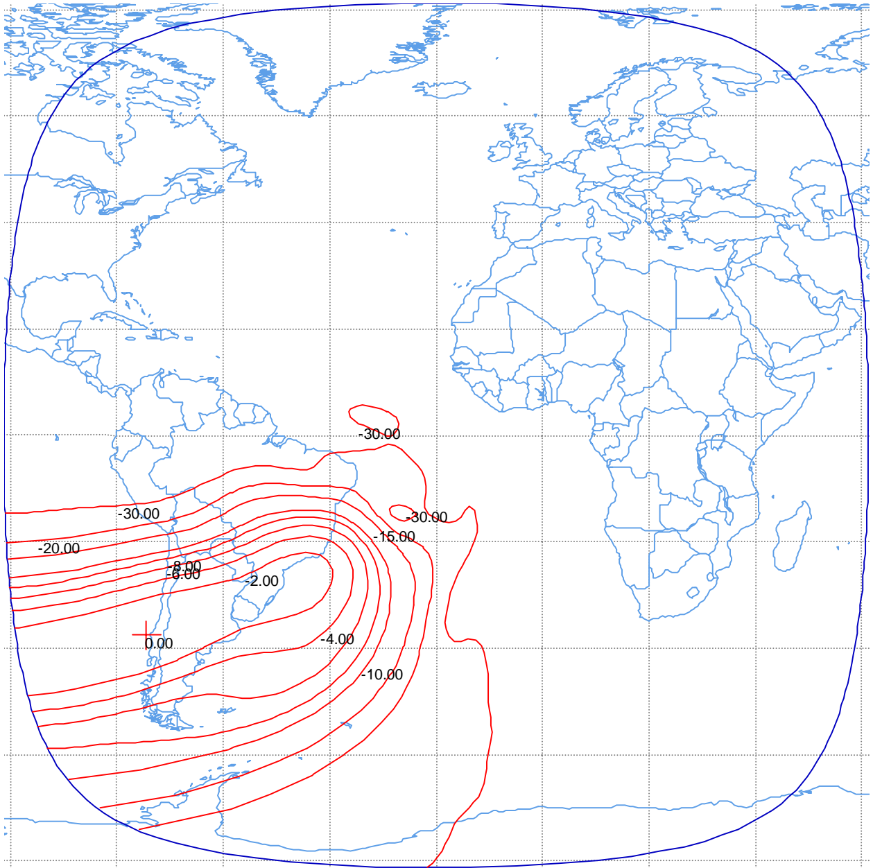
Figure B-12. South West Zone Downlink Beam Peak EIRP = 43.8 dBW Peak Beam Gain = 32.1 dBi Polarization LHCP Schedule S beam designator: SWZD
