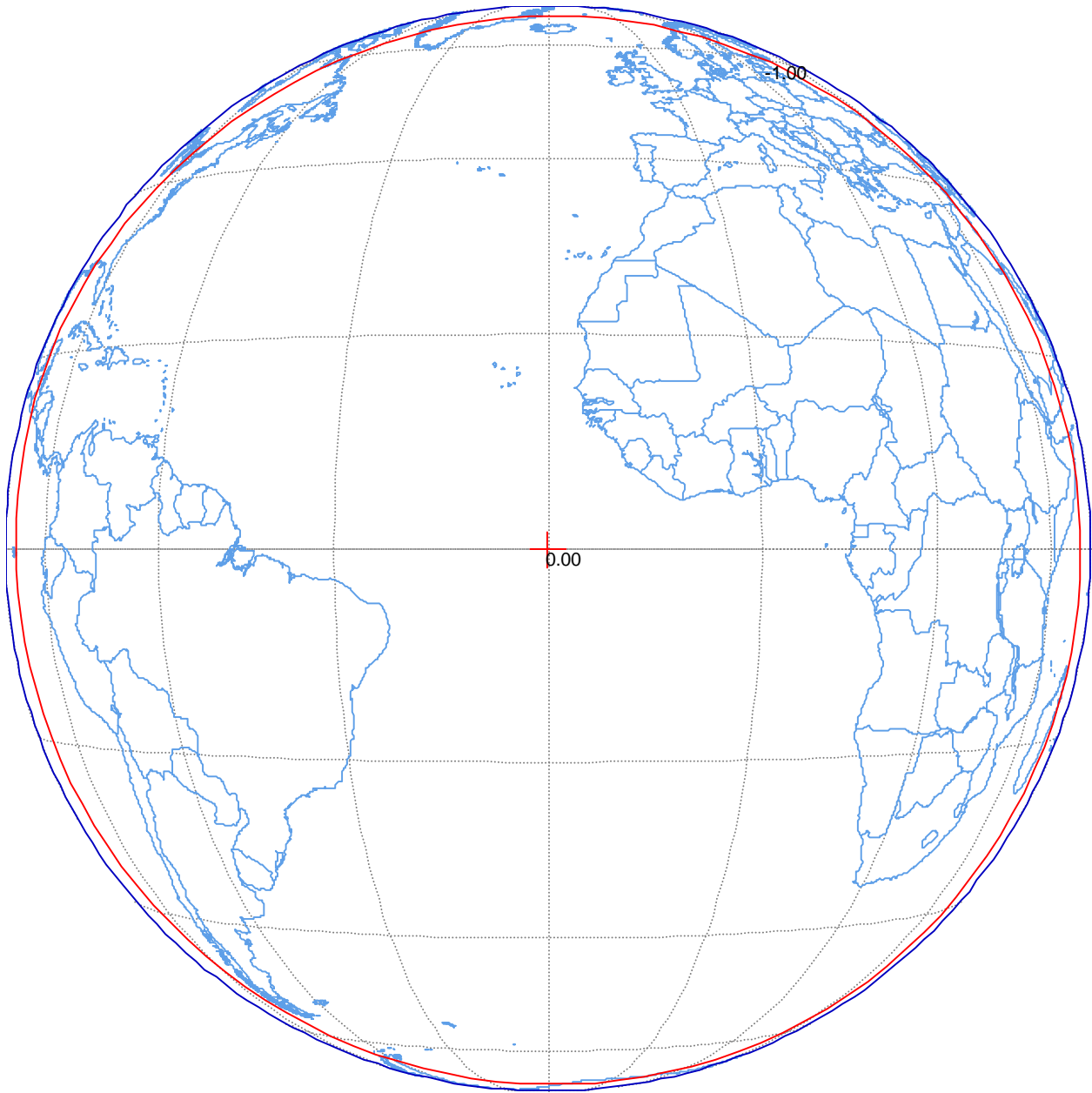
Figure B-25. C-band Tracking Beacon Earth Facing Transmit Horn 14 Maximum EIRP = 11 dBW Maximum transmit gain = 11.3 dBi Polarization Vertical Linear Schedule S beam designator: BNC
