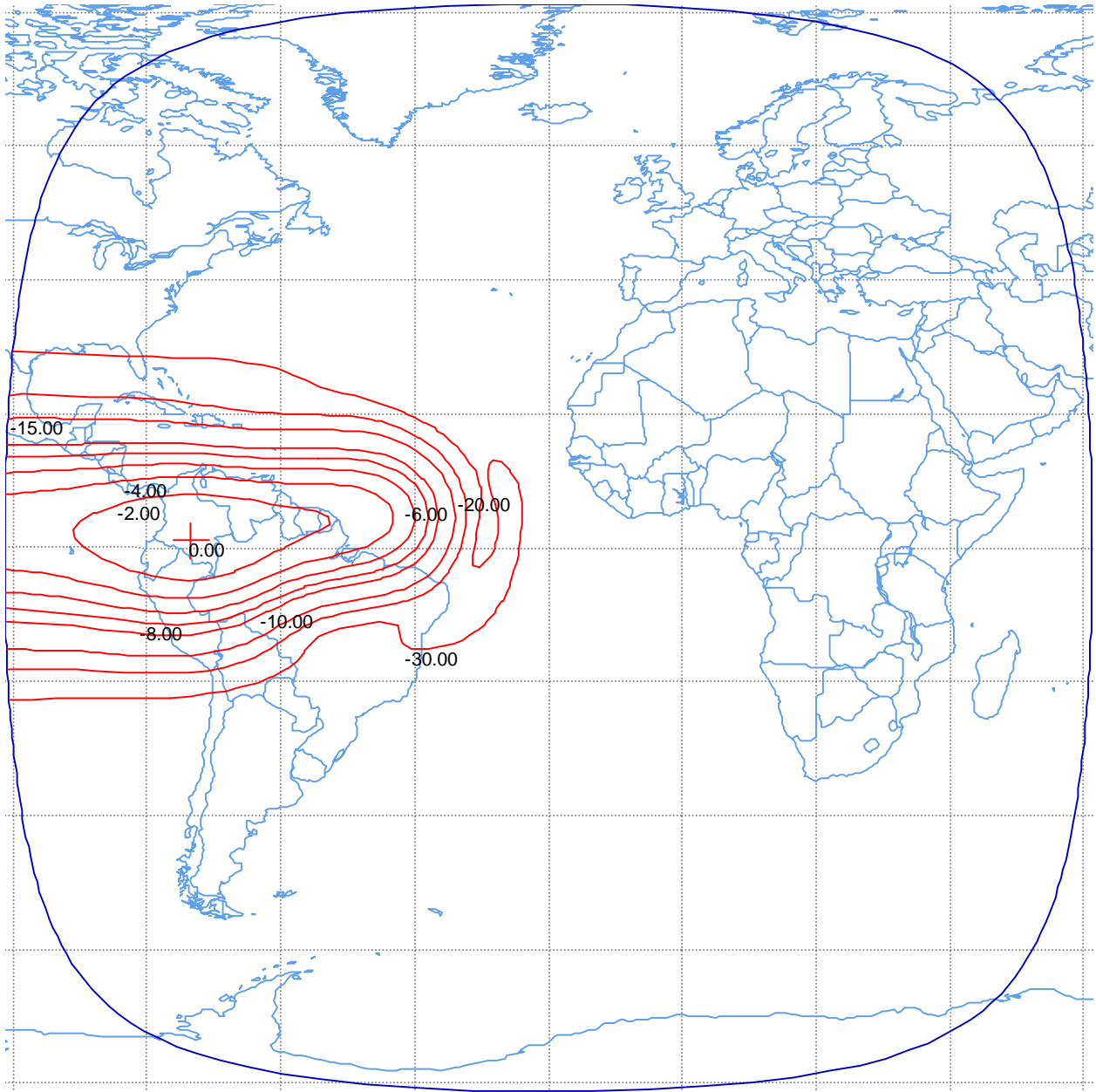
Figure B-16. Mid West Zone Downlink Beam Peak EIRP = 42.5 dBW Peak Beam Gain = 33.3 dBi Polarization LHCP Schedule S beam designator: MWZD
