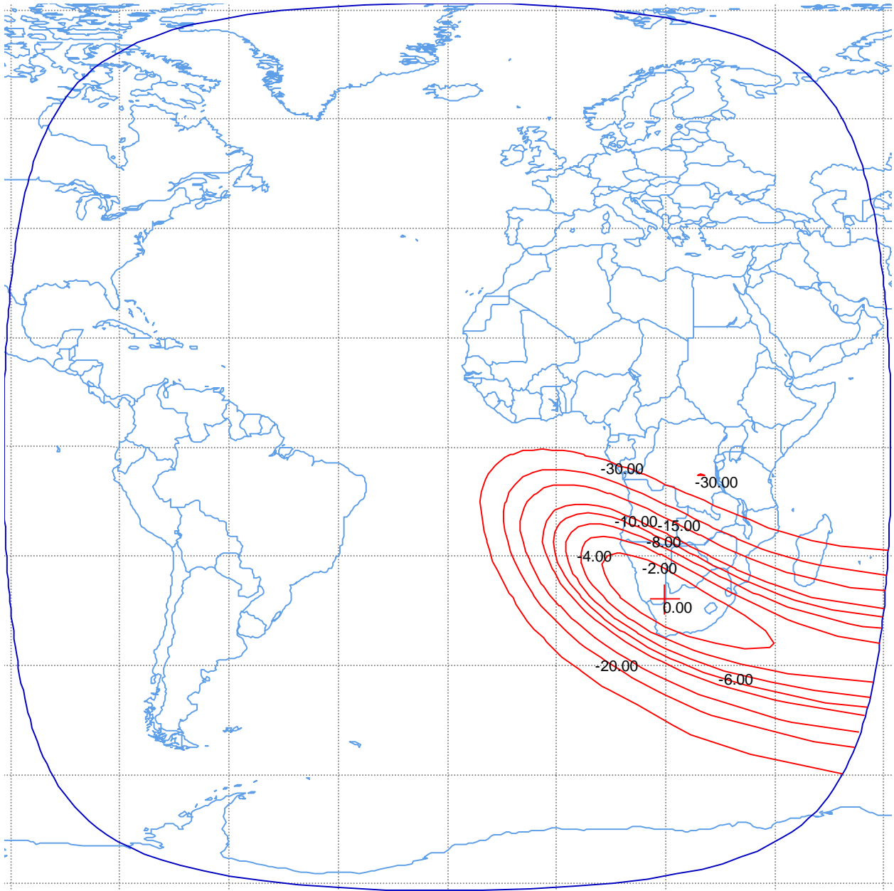
Figure B-27. Ku-band Tracking Beacon with Spot 2 antenna Maximum EIRP = 9 dBW Maximum transmit gain = 36.9 dBi Polarization Linear Vertical or Horizontal Schedule S beam designator: BNK3
