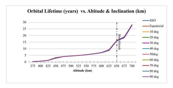
Spire has also run an analysis measuring dwell times across the entire solar cycle to ensure that changes in launch schedule do not cause Spire to violate Requirement 4.6.1 at a maximum deployment apogee of 650 km.
