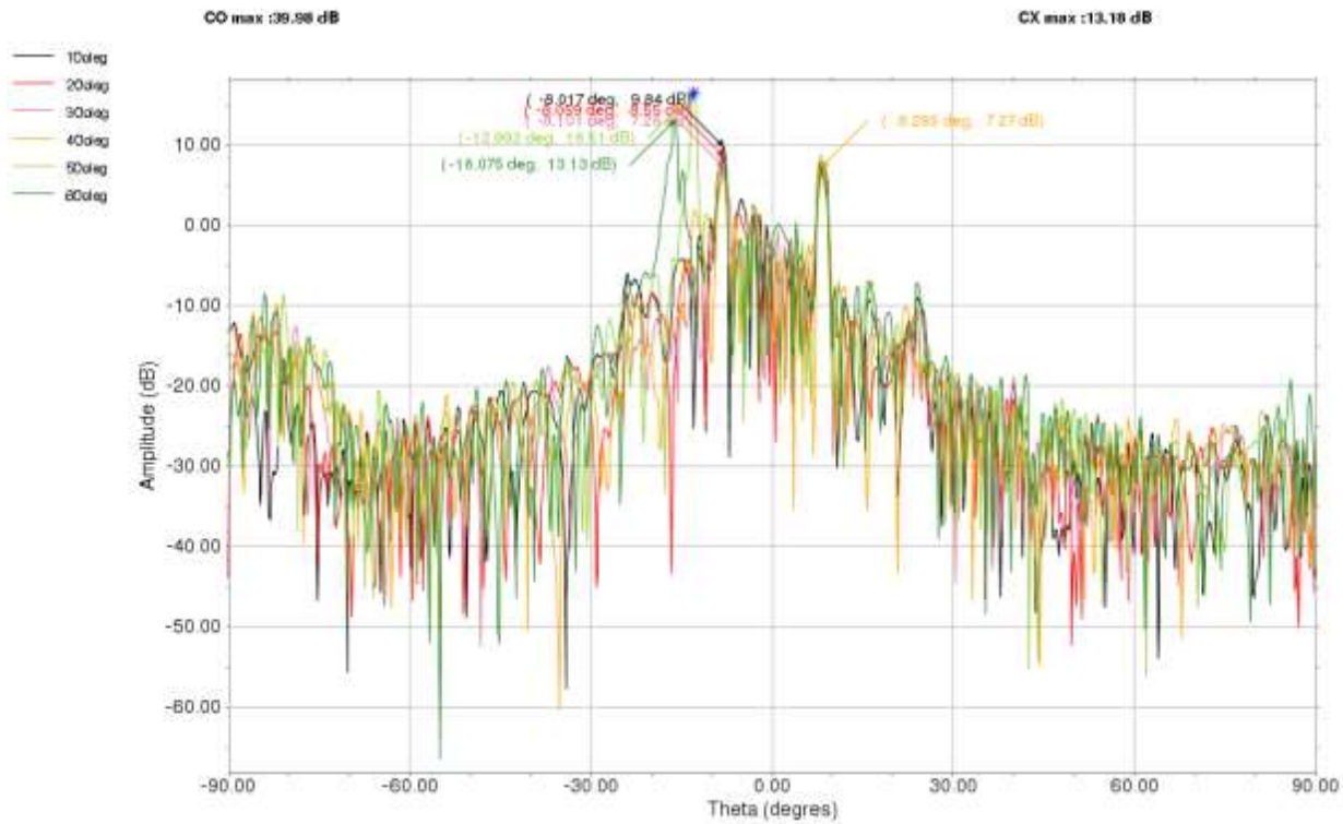
BEAM GW No6 - EQUAT. CUTS [Theta +/-90deg , Phi 10 to 60deg] at 17305.0 MHz rhcp
