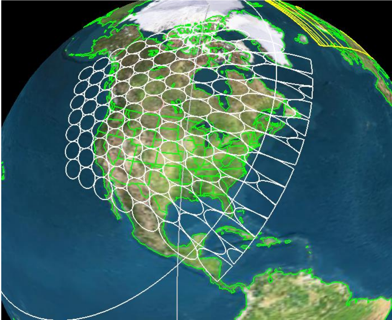
Figure 5 Satellite transmit and receive user link beam array at the start (most Westward end) of the West North America active arc. The large circle is the 20-degree elevation angle contour to the satellite. The beams terminate in this illustration at 10 degrees elevation angle rather than at 0 degrees. Only those beams serving the Western United States West of the vertical line at approximately 94 degrees West are active on this satellite. The East North America active arc serves the United States East of the vertical line.
