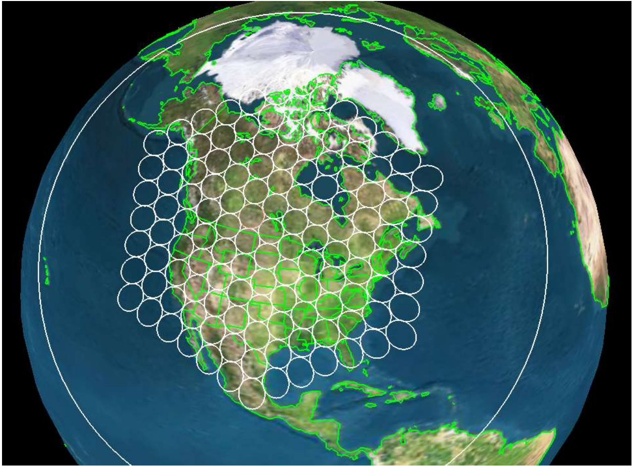
Figure 5 Satellite beam array at the end of the West North American active arc, also showing the 20 degree elevation angle contour to the satellite.
