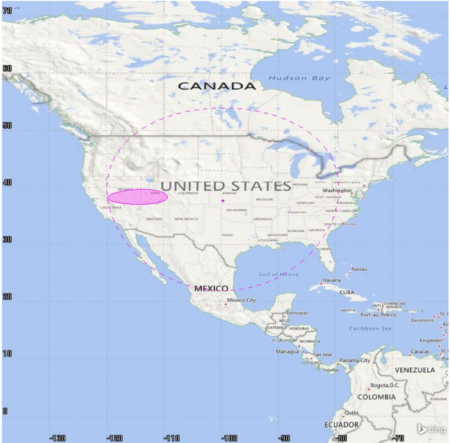
Figure 4: Single Kepler satellite half power beam width visible on the ground when steered to a 64 degree angle off boresight.
