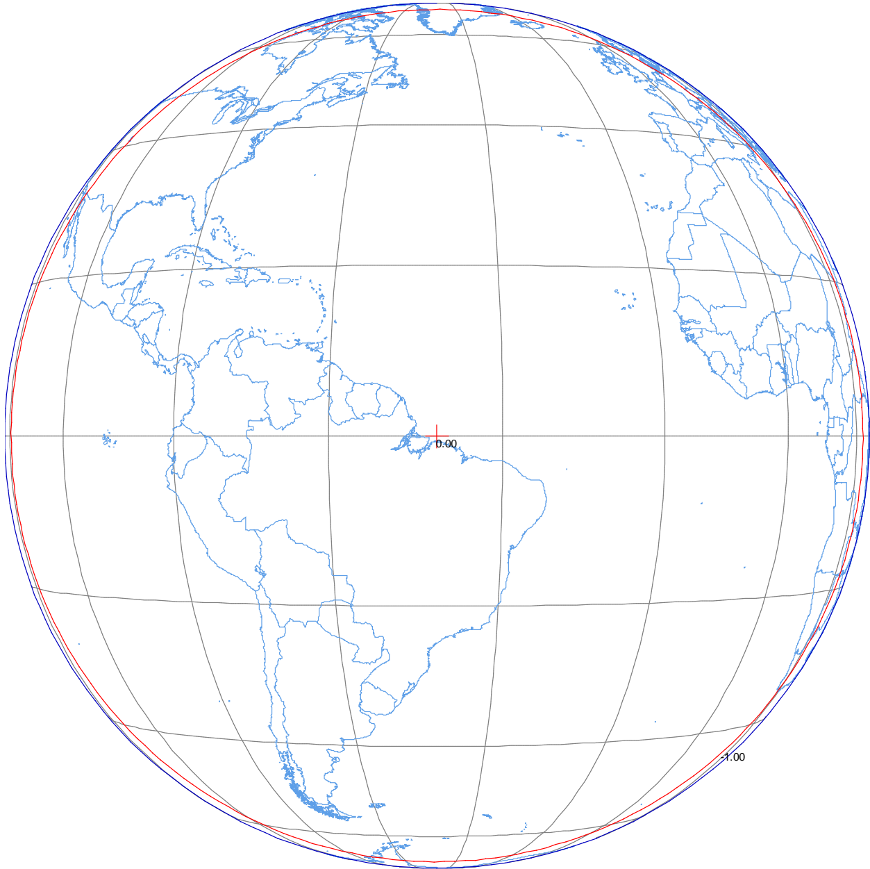
Figure A-5. Command Carrier Earth Facing Receive Horn 4 Maximum receive gain = 10.3 dBi Command Threshold Flux Density = -90 dBW/m 2 Polarization LHCP Schedule S beam designators: CMD
