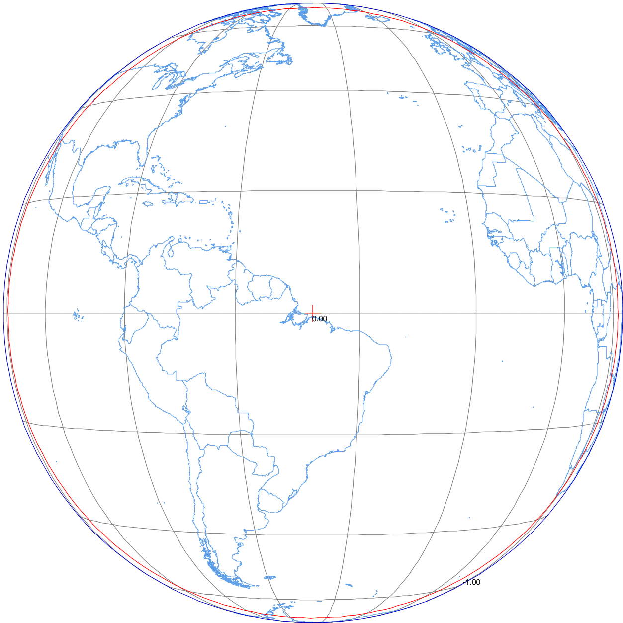
Figure A-7. C-band Tracking Beacon Earth Facing Transmit Horn 6 Maximum EIRP = 11 dBW Maximum transmit gain = 11.3 dBi Polarization Vertical Linear Schedule S beam designators: BNC
