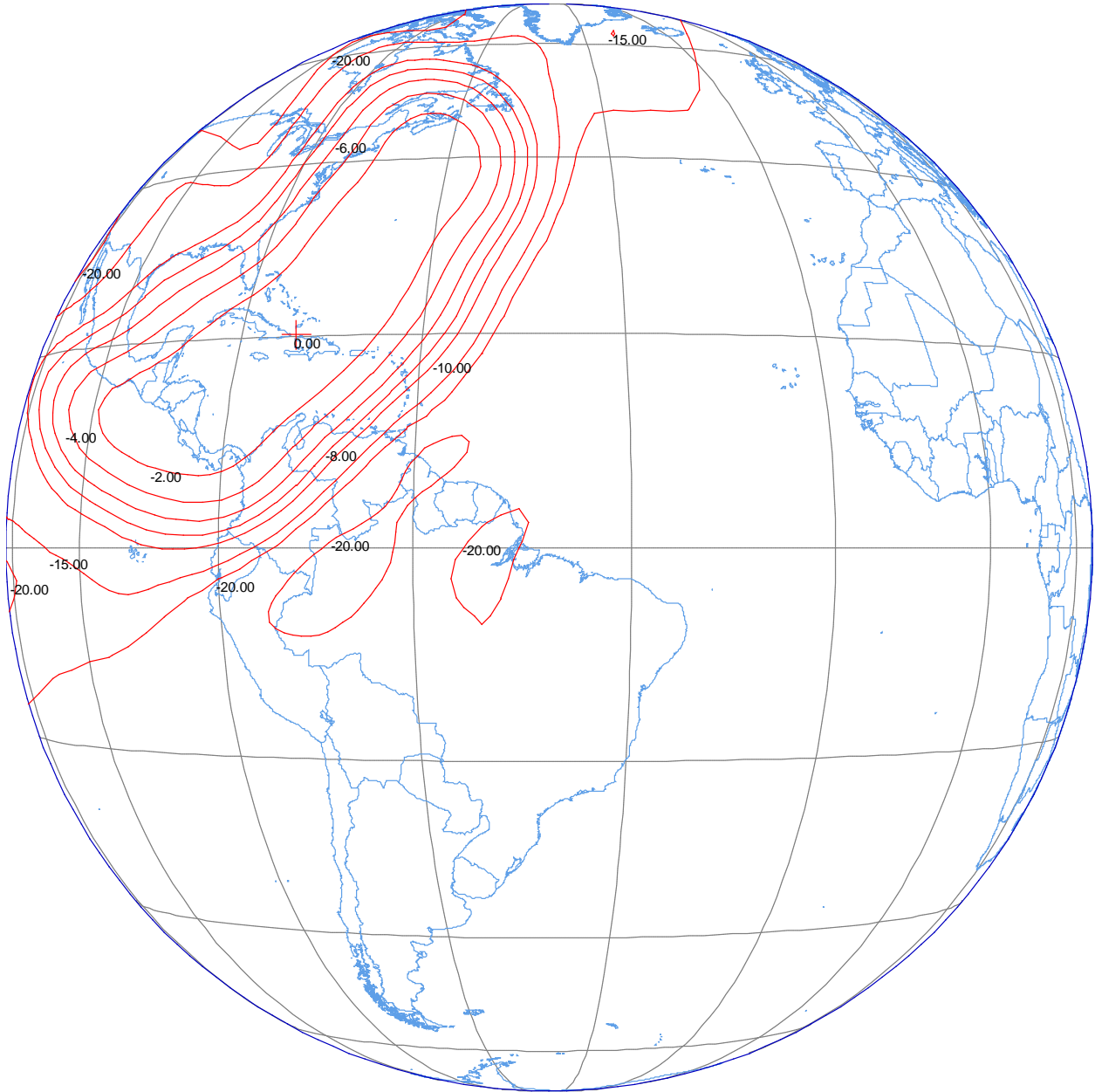
Figure A-8. Ku-band Tracking Beacon Antenna Maximum EIRP = 9 dBW Maximum transmit gain = 32.3 dBi Polarization Horizontal Linear Schedule S beam designators: BNK
