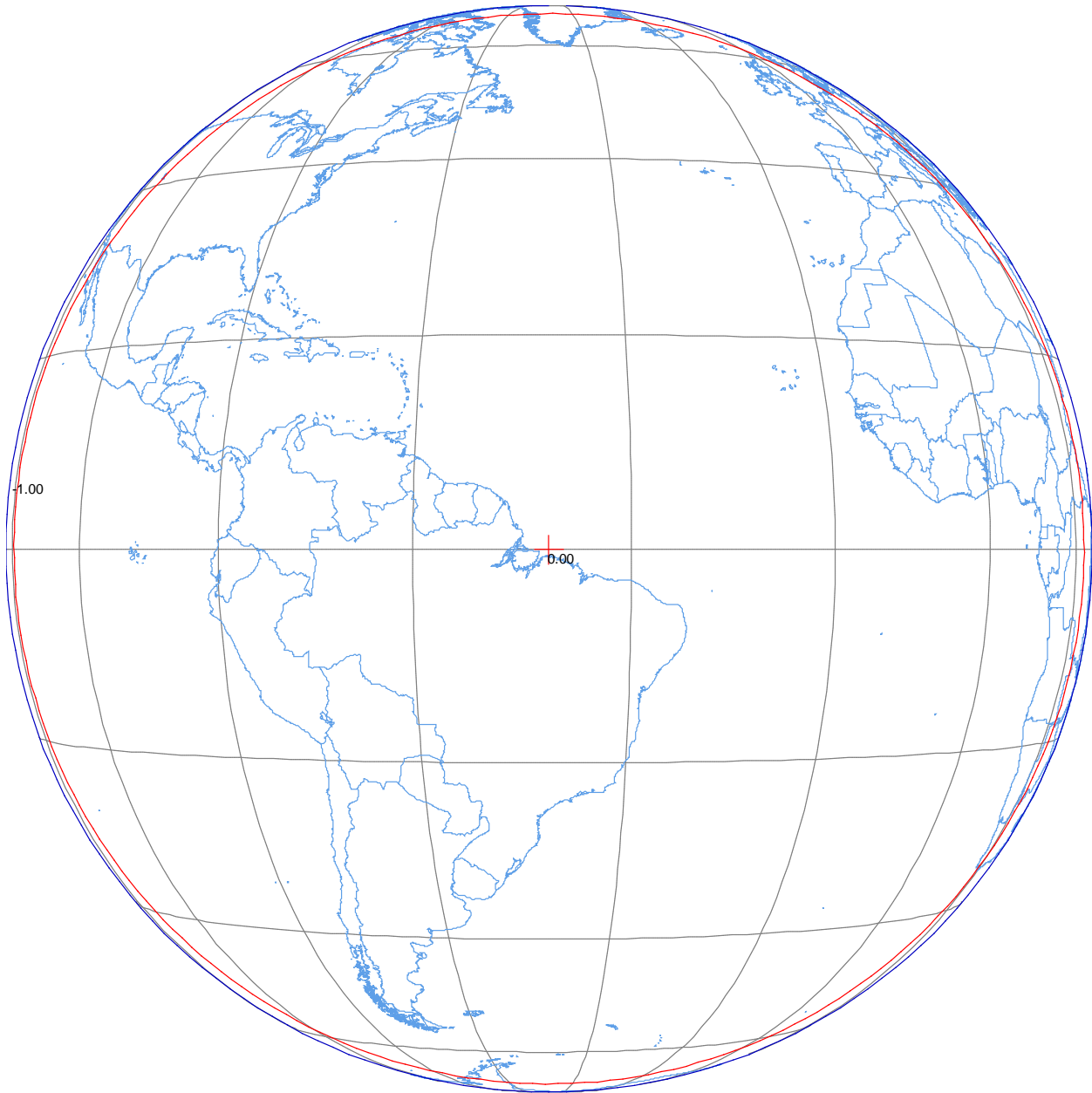
Figure A-6. Telemetry Carrier Earth Facing Transmit Horn 5 Maximum EIRP = 10 dBW Maximum transmit gain = 11.3 dBi Polarization RHCP Schedule S beam designators: TLM
