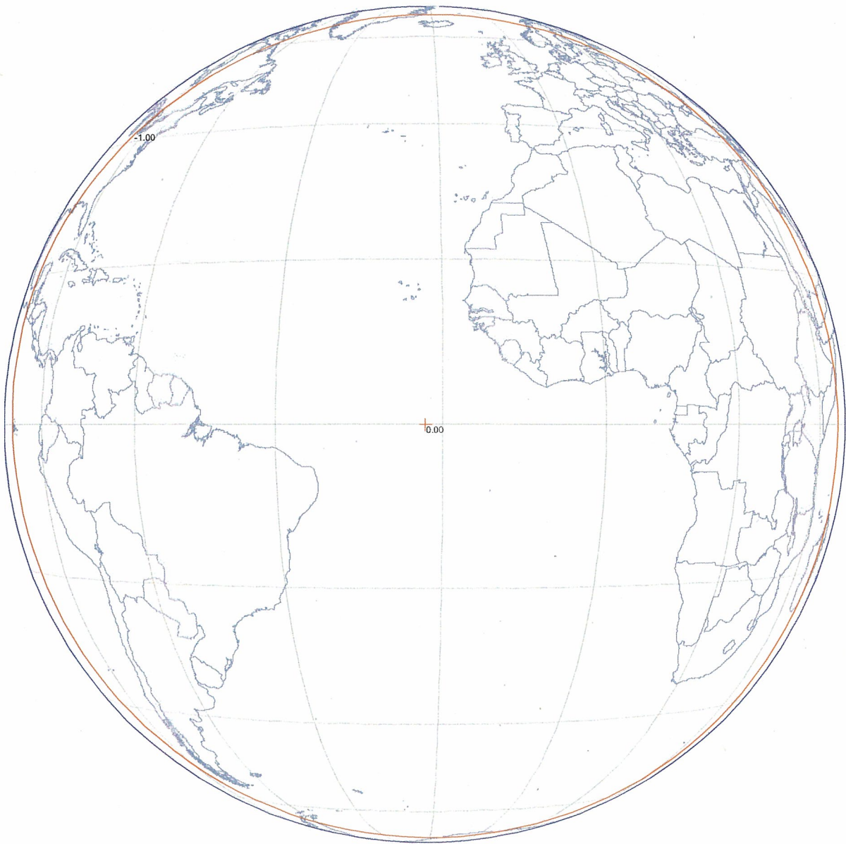
Figure B-17. Telemetry Carrier Earth Facing Omni Antenna (Emergency) 13 Maximum EIRP = 21 dBW Maximum transmit gain = 8 dBi Polarization LHCP and RHCP Schedule S beam designator: OMNI
