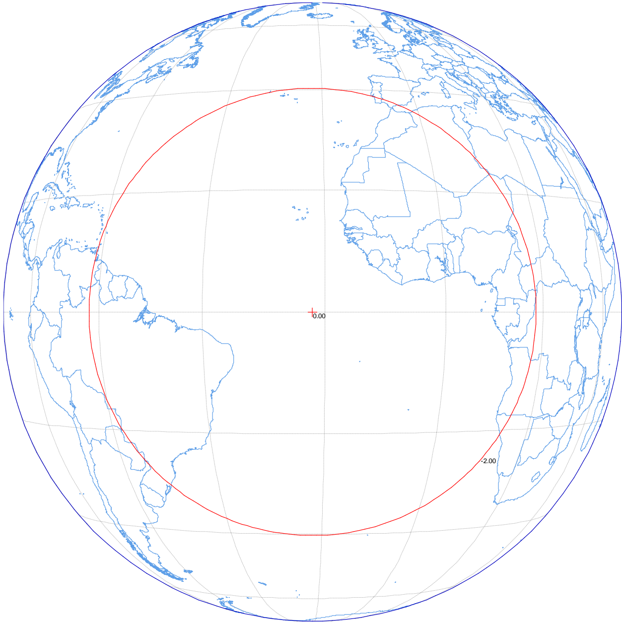
Figure B-16. Telemetry Carrier Earth Facing Transmit Horn 12 Maximum EIRP = 16 dBW Maximum transmit gain = 22 dBi Polarization LHCP and RHCP Schedule S beam designator: TLM
