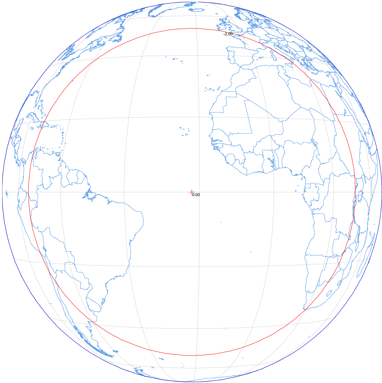
Figure B-18. C-band Tracking Beacon Earth Facing Transmit Horn 14 Maximum EIRP = 19.2 dBW Maximum transmit gain = 19.6 dBi Polarization Vertical Linear Schedule S beam designator: BNC
