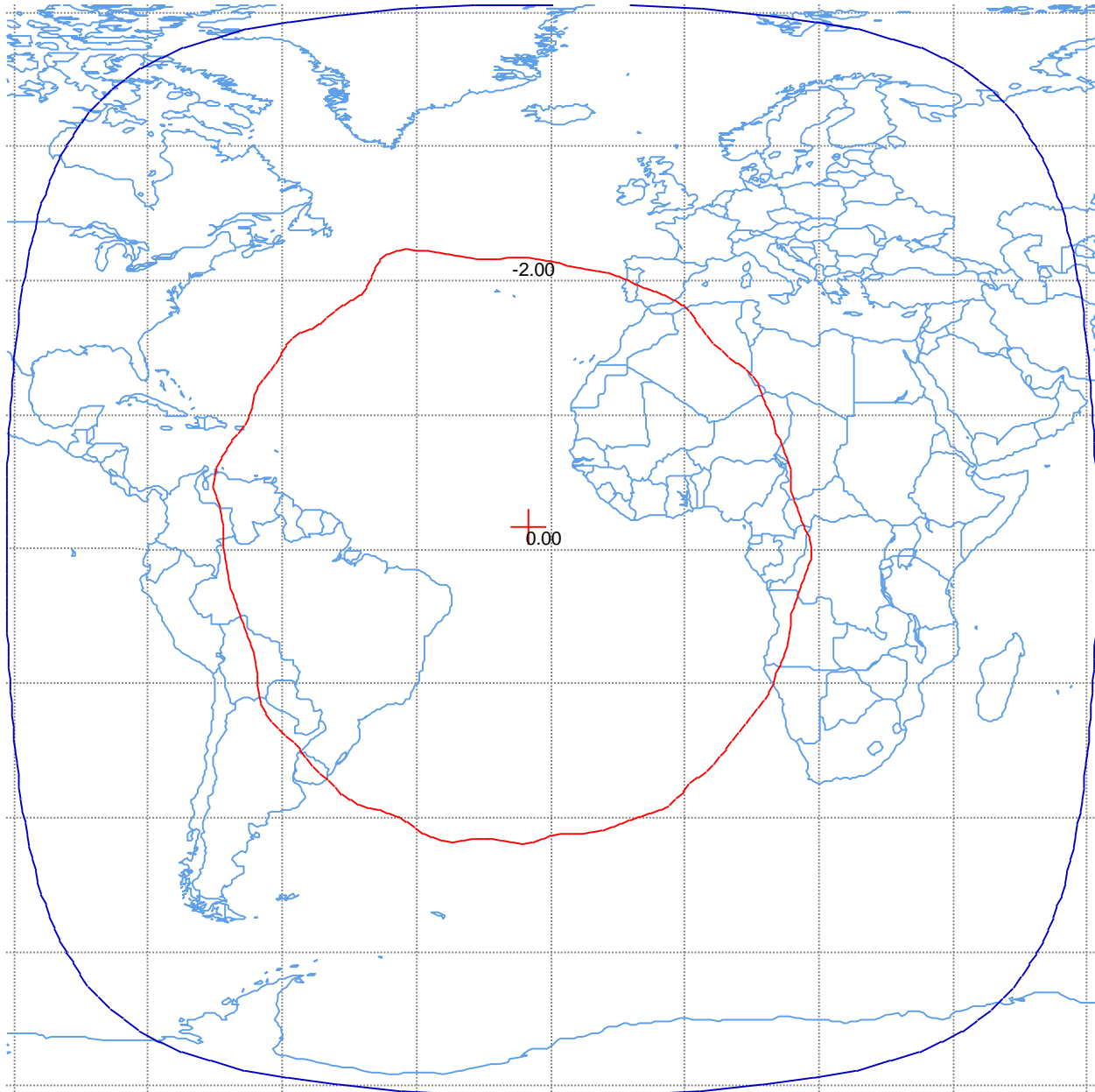
Figure B-1. Global Uplink Beam Peak G/T = -6.3 dB/K Peak Beam Gain = 21.1dBi Min. Saturation Flux Density = -94dBW/m 2 Polarization LHCP and RHCP Schedule S beam designators: GBAU and GBBU 6
