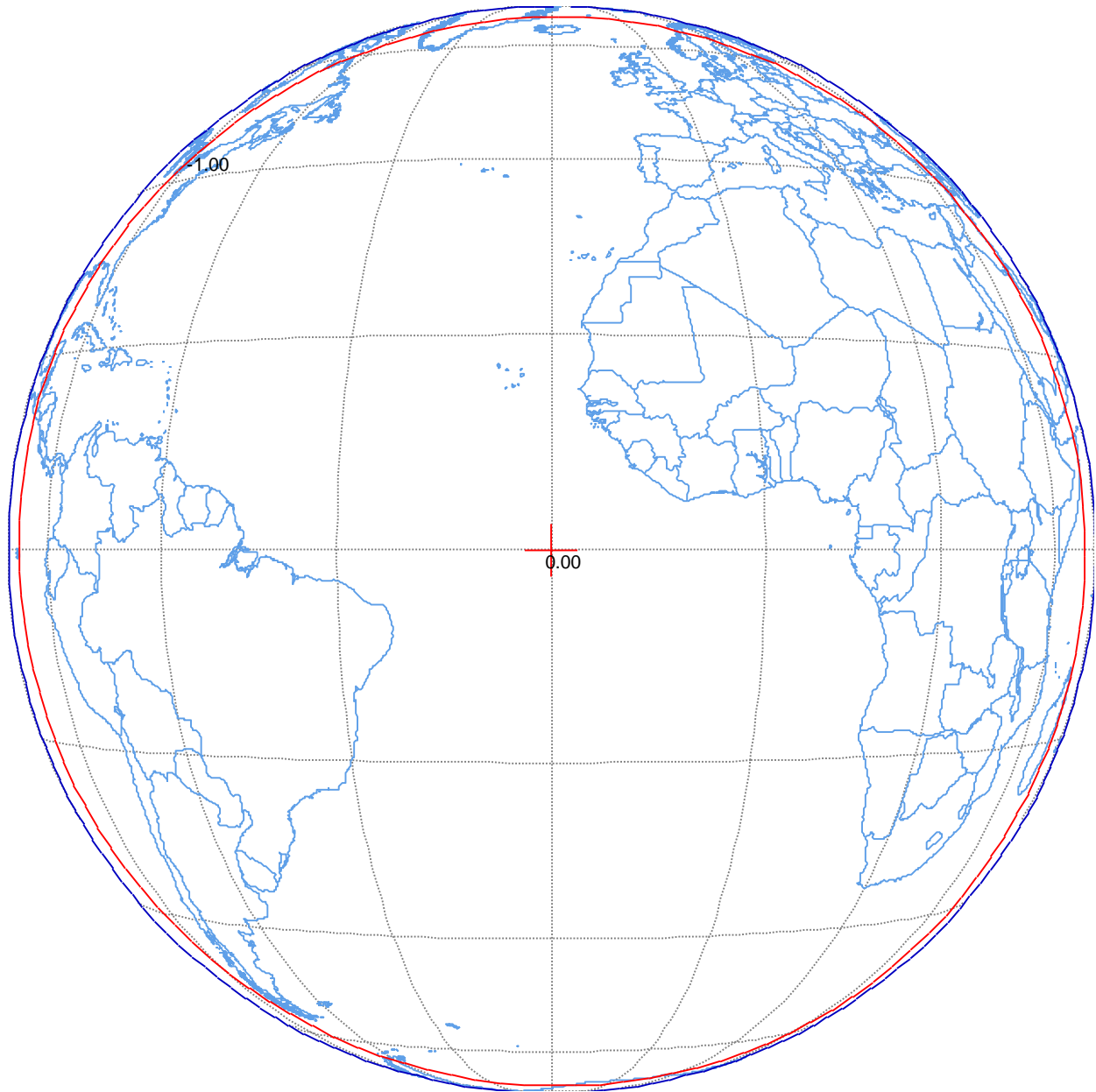
Figure B-23. Command Carrier Earth Facing Receive Horn 8 Maximum receive gain = 11dBi Command Threshold Flux Density = -89dBW/m 2 Polarization Vertical Linear Schedule S beam designator: CMD
