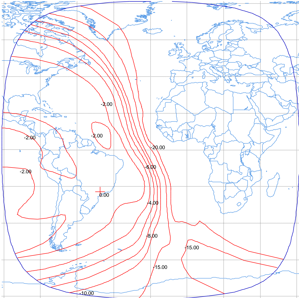
Figure B-3. West Hemi Uplink Beam Peak G/T = -2.3 dB/K Peak Beam Gain = 25.8dBi Min. Saturation Flux Density = -96dBW/m 2 Polarization LHCP and RHCP Schedule S beam designator: WHAU and WHBU
