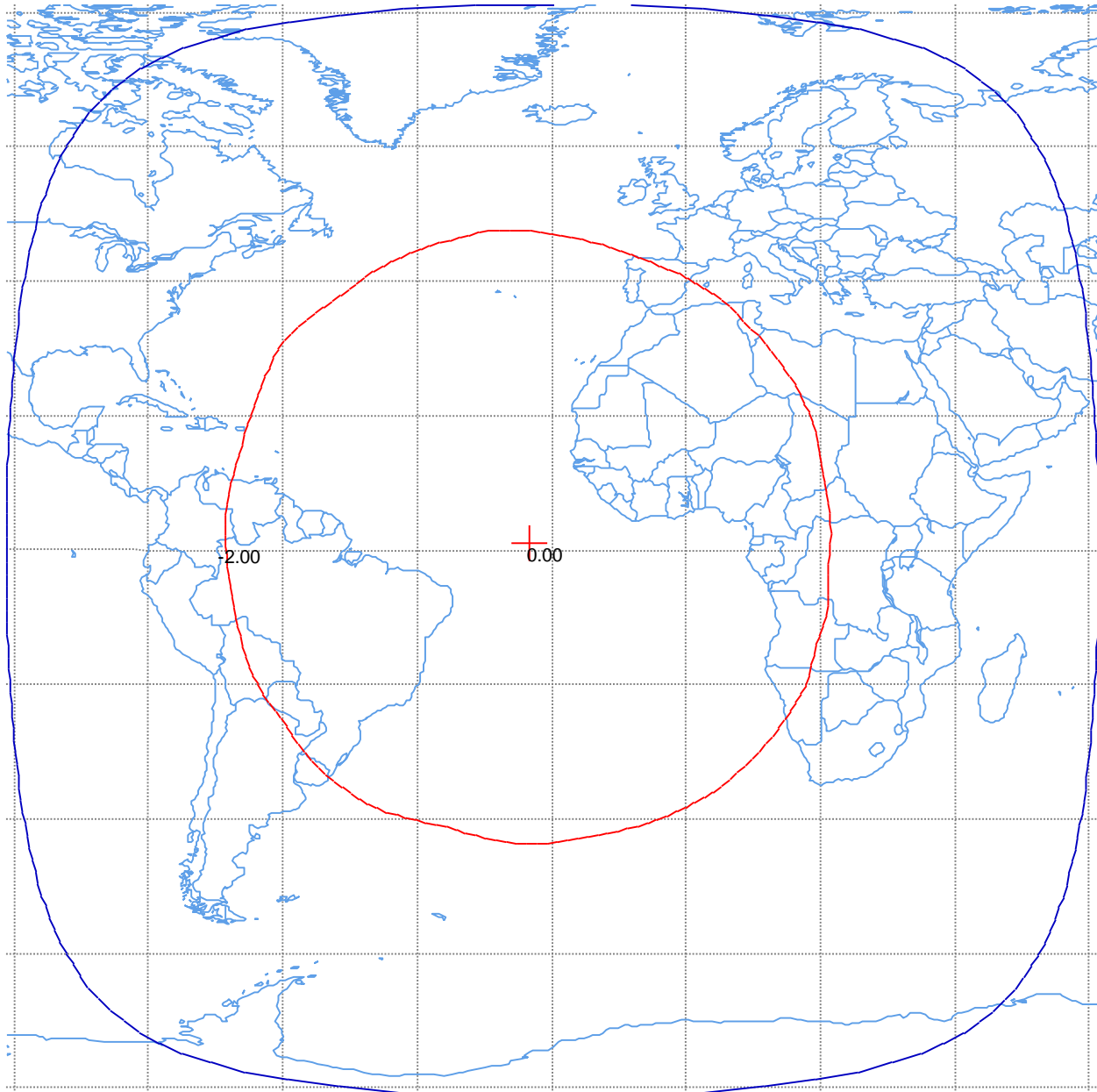
Figure B-2. Global Downlink Beam Peak EIRP = 36.1dBW Peak Beam Gain = 20.8dBi Polarization RHCP and LHCP Schedule S beam designators: GBAD and GBB 7
