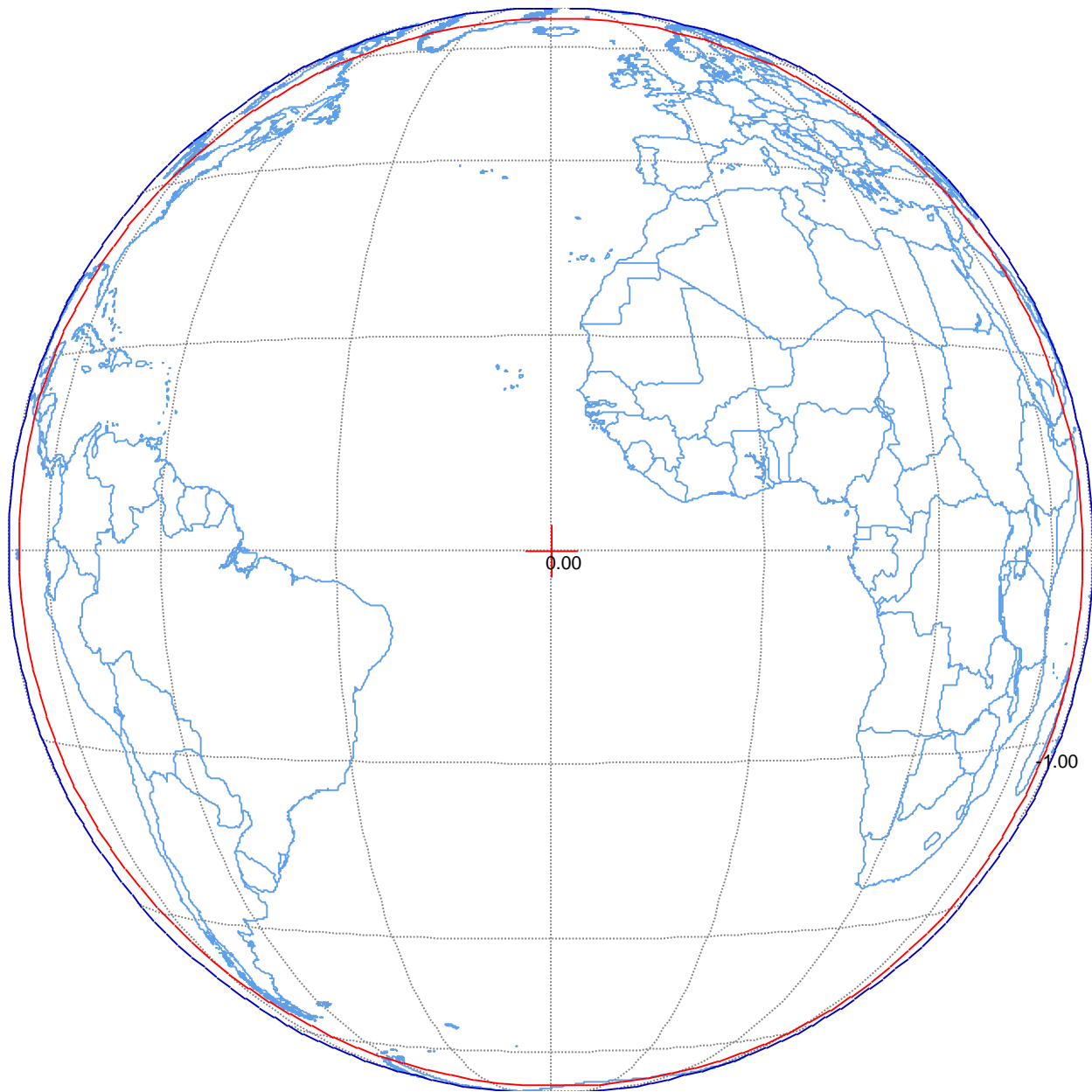
Figure B-26. Ku-band Tracking Beacon Earth Facing Transmit Horn 11 Maximum EIRP = 9dBW Maximum transmit gain = 11dBi Polarization Horizontal Linear Schedule S beam designator: BNK
