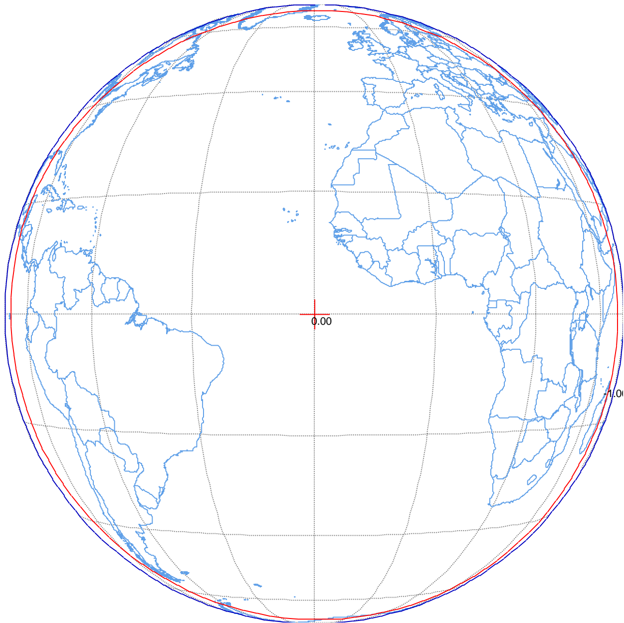
Figure B-24. Telemetry Carrier Earth Facing Transmit Horn 9 Maximum EIRP = 9dBW Maximum transmit gain = 11dBi Polarization Horizontal Linear Schedule S beam designator: TLM
