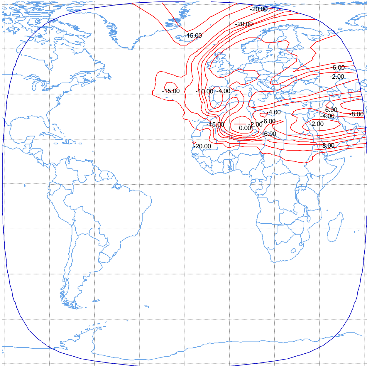
Figure B-11. Europe/Middle East Uplink Beam Peak G/T = 6.6 dB/K Peak Beam Gain = 34.7 dBi Min. Saturation Flux Density = -98 dBW/m 2 Polarization Vertical and Horizontal Linear Schedule S beam designators: EUAU and EUBU
