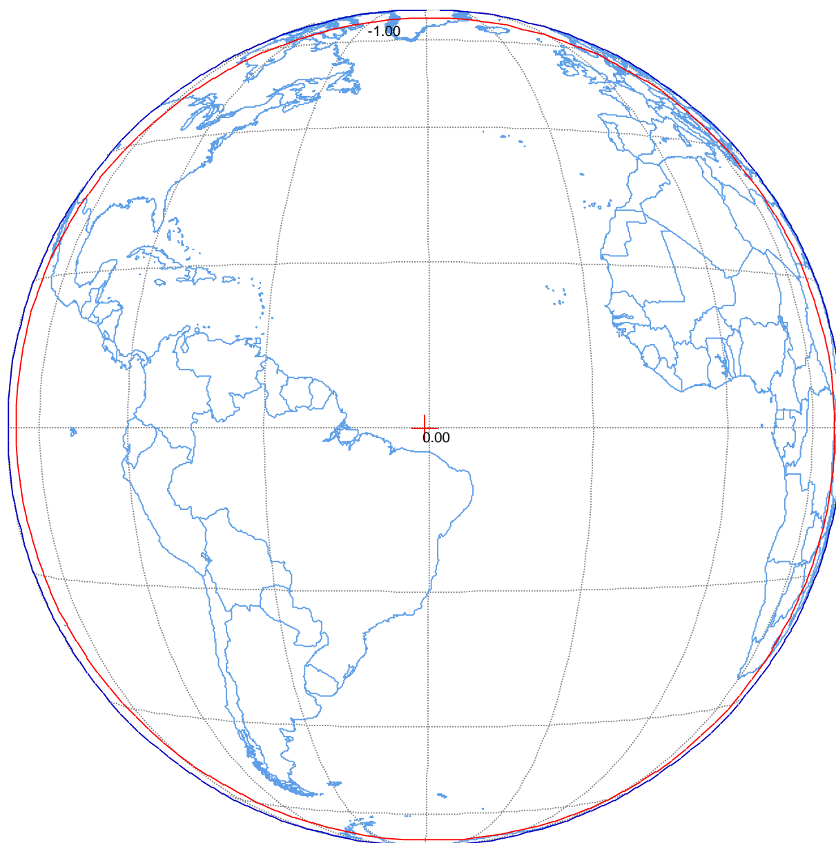
Figure B-9. Command Carrier Earth Facing Receive Horn 6 Maximum receive gain = 10.3 dBi Command Threshold Flux Density = -90 dBW/m 2 Peak Beam Gain = 32.2 dBi Polarization LHCP Schedule S beam designators: CMD
