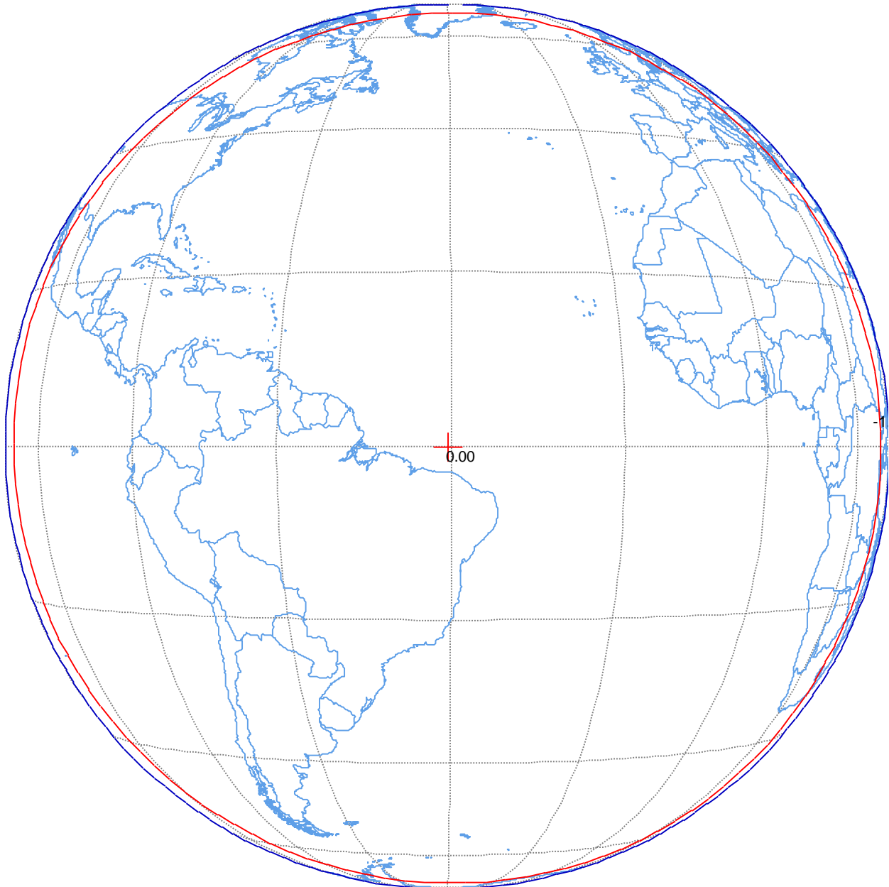
Figure B-10. Telemetry Carrier Earth Facing Transmit Horn 7 Maximum EIRP = 10 dBW Maximum transmit gain = 11.3 dBi Polarization RHCP Schedule S beam designators: TLM
