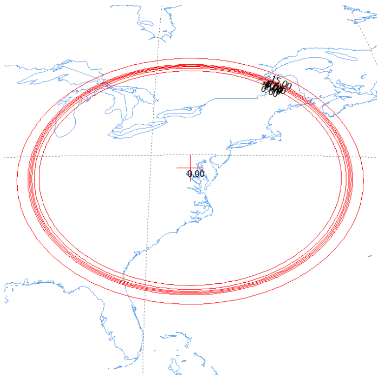
Figure 15: LD1R Antenna Beam Projection over District of Columbia, USA (Scan Angle)
