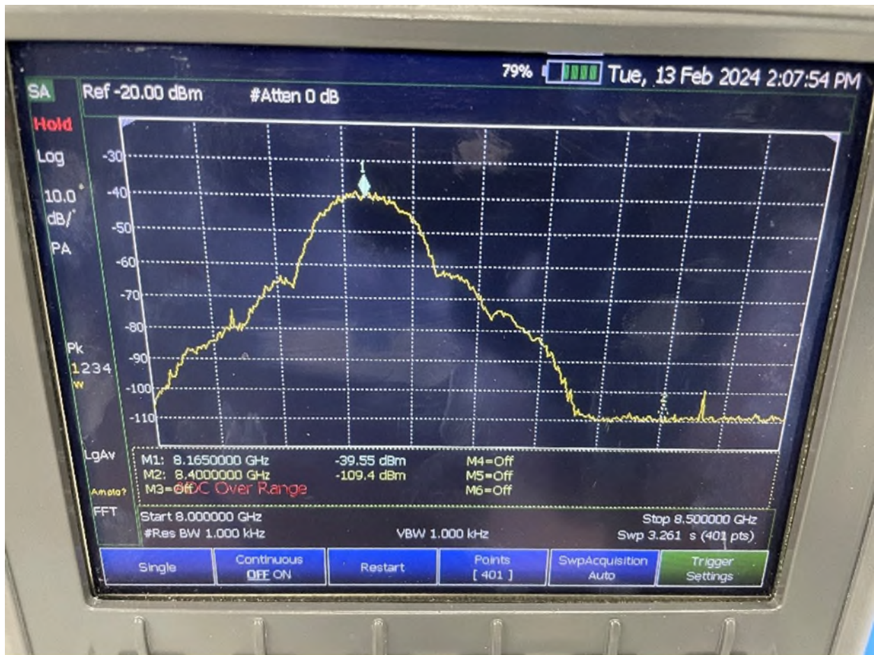
Figure 2 X-Band Payload #1 Downlink - Out of Band Emissions Measurement
