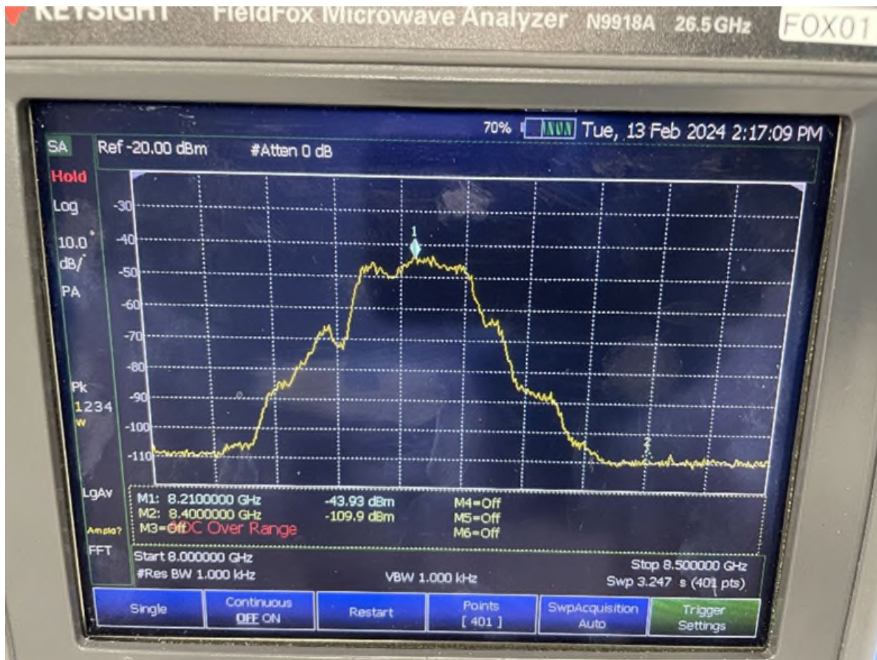
Figure 3 X-Band Payload #2 Downlink - Out of Band Emissions Measurement
