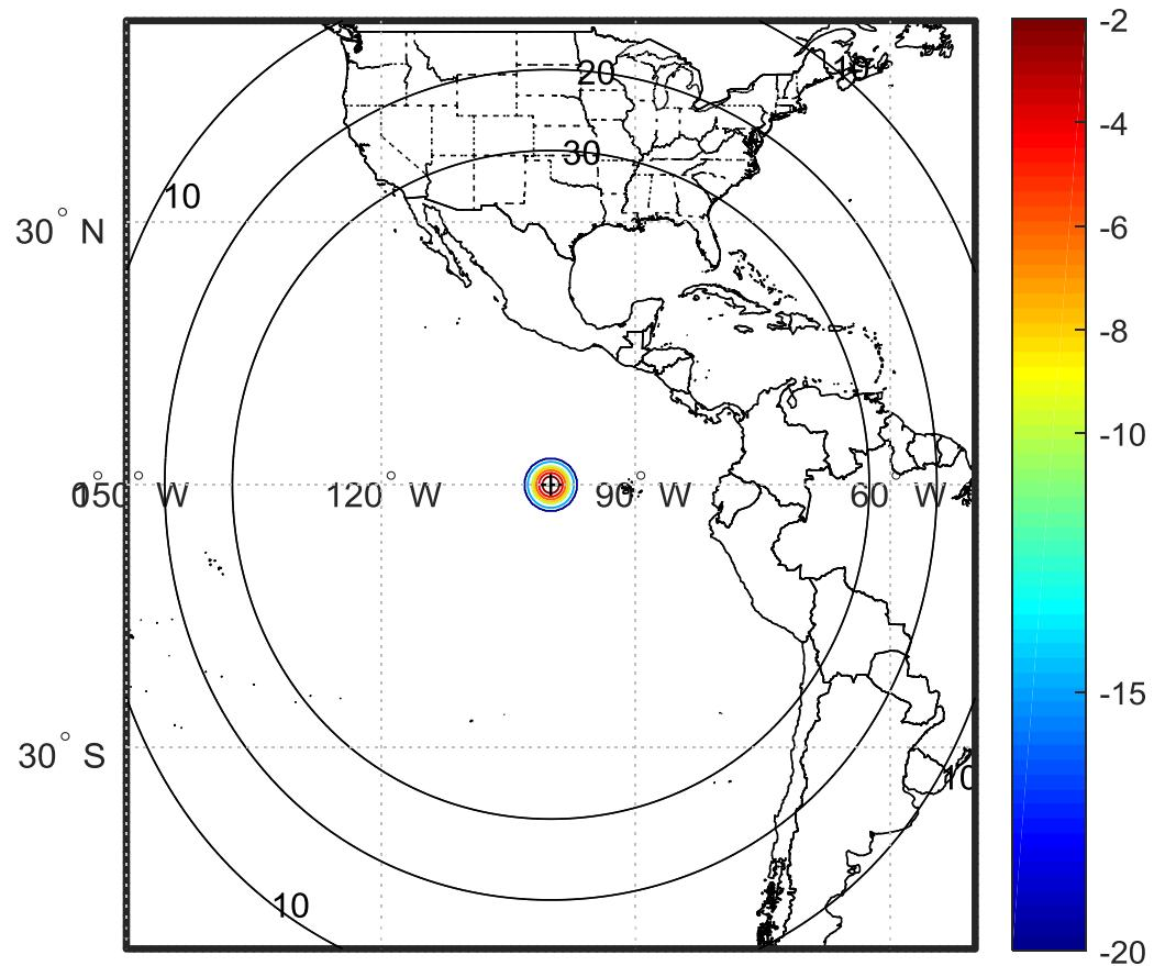
MEO TX beam 30-degree elevation angle
