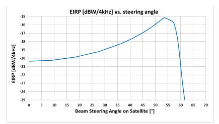
Figure A.3.1-1. EIRP Density Variation by Beam Steering Angle (540 km)
