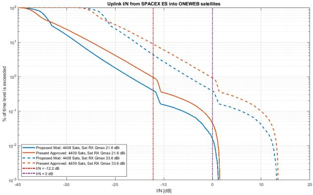
Figure A1-7. Uplink Comparison for Various OneWeb Antennas at 35°N (Ku-band)
