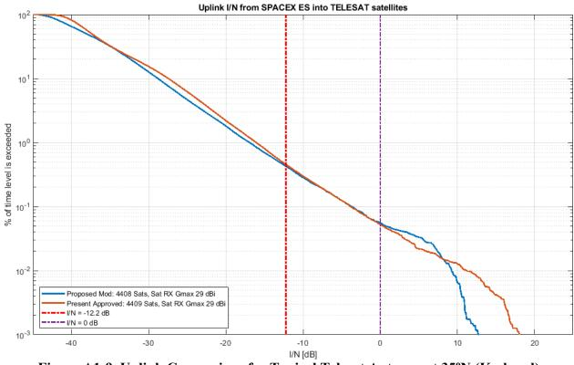
Figure A1-9. Uplink Comparison for Typical Telesat Antenna at 35°N (Ka-band)
