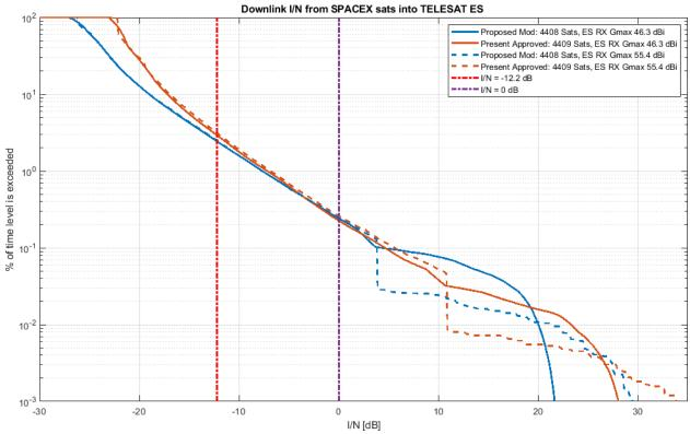
Figure A1-2. Downlink Comparison for Various Telesat Antennas at 35°N (Ka-band)
