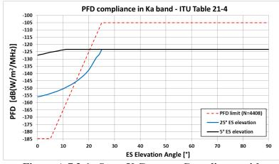
Figure A.7.2-1. SpaceX Gateway Compliance with Downlink PFD Limits in the 17.7-19.3 GHz Band
