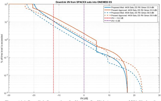
Figure A1-1. Downlink Comparison for Various OneWeb Antennas at 35°N (Ku-band)
