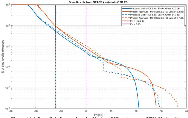
Figure A1-6. Downlink Comparison for Various O3B Antennas at 75°N (Ka-band)
