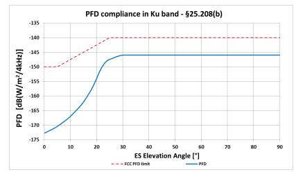
Figure A.7.1-1. Compliance with Downlink PFD Limits in the 10.7-11.7 GHz Band (540 km)
