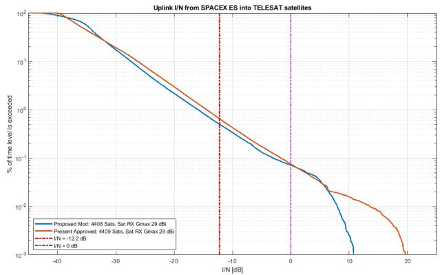
Figure A1-10. Uplink Comparison for Typical Telesat Antenna at 75°N (Ka-band)
