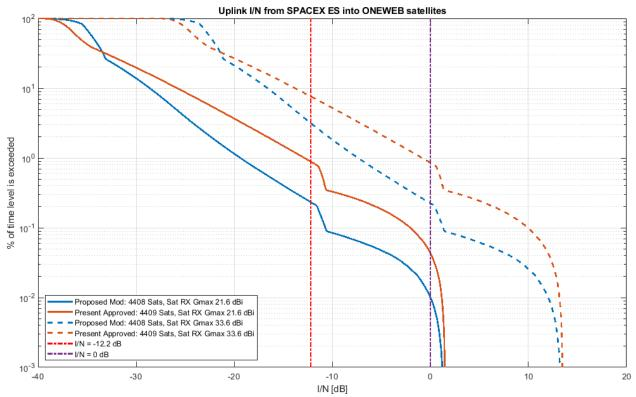
Figure A1-8. Uplink Comparison for Various OneWeb Antennas at 75°N (Ku-band)
