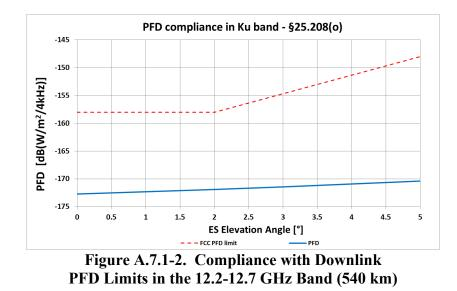
Operations at this lowest shell provide a worst-case PFD scenario, yet still remain compliant. Accordingly, all Ku-band downlink transmissions from SpaceX satellites operating in the modified constellation will comply with all applicable Commission and ITU PFD limits.
