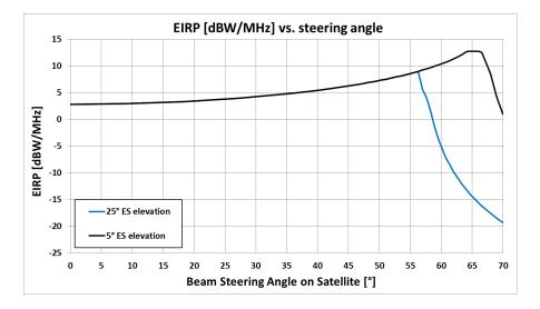
Figure A.3.2-1: EIRP Density Variation by Beam Steering Angle
