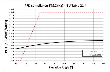
Figure A.7.2-2. SpaceX TT&C Compliance with Downlink PFD Limits in the 17.7-19.3 GHz Band
