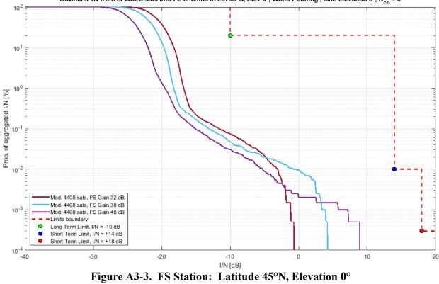
Downlink I/N from SPACEX sats into FS antenna at Lat 45°N, Elev 0°, Worst Pointing , Min. Elevation 5°, N<sub>co</sub> = 8
