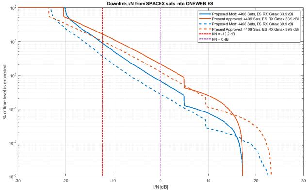
Figure A1-2. Downlink Comparison for Various OneWeb Antennas at 75°N (Ku-band)
