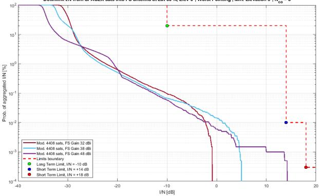
Downlink I/N from SPACEX sats into FS antenna at Lat 60°N, Elev 0°, Worst Pointing , Min. Elevation 5°, N<sub>co</sub> = 8
