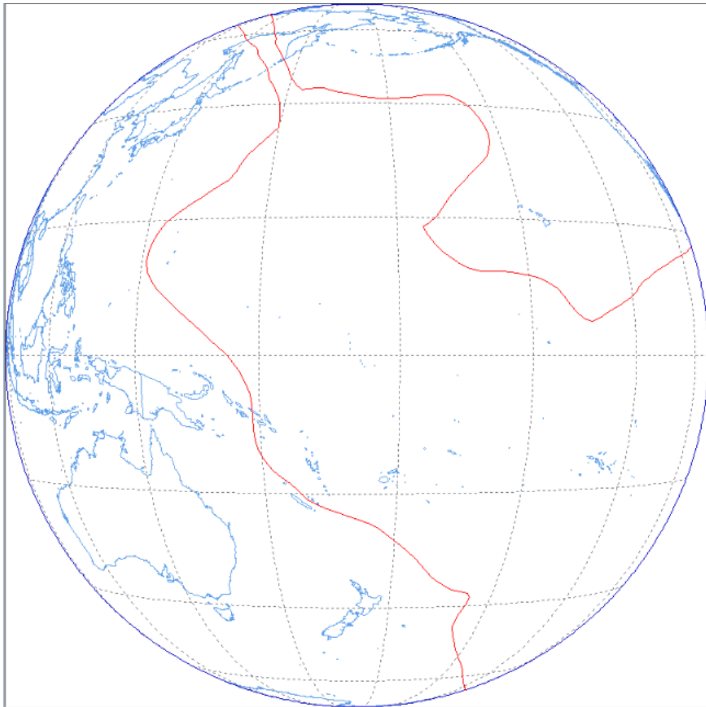
Figure 1 C-band POR Coverage from 174°E.L.
