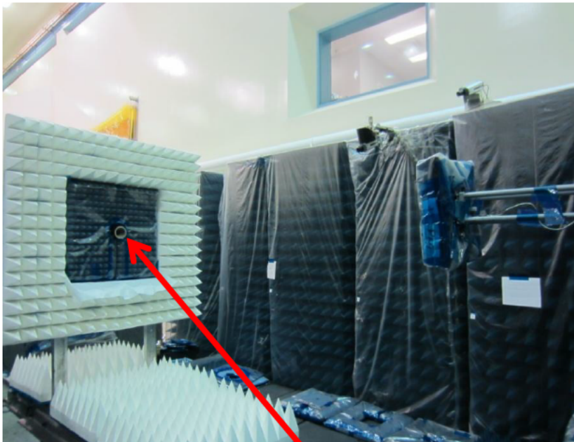
R Band feed assembly during radiation pattern measurement at MDA
